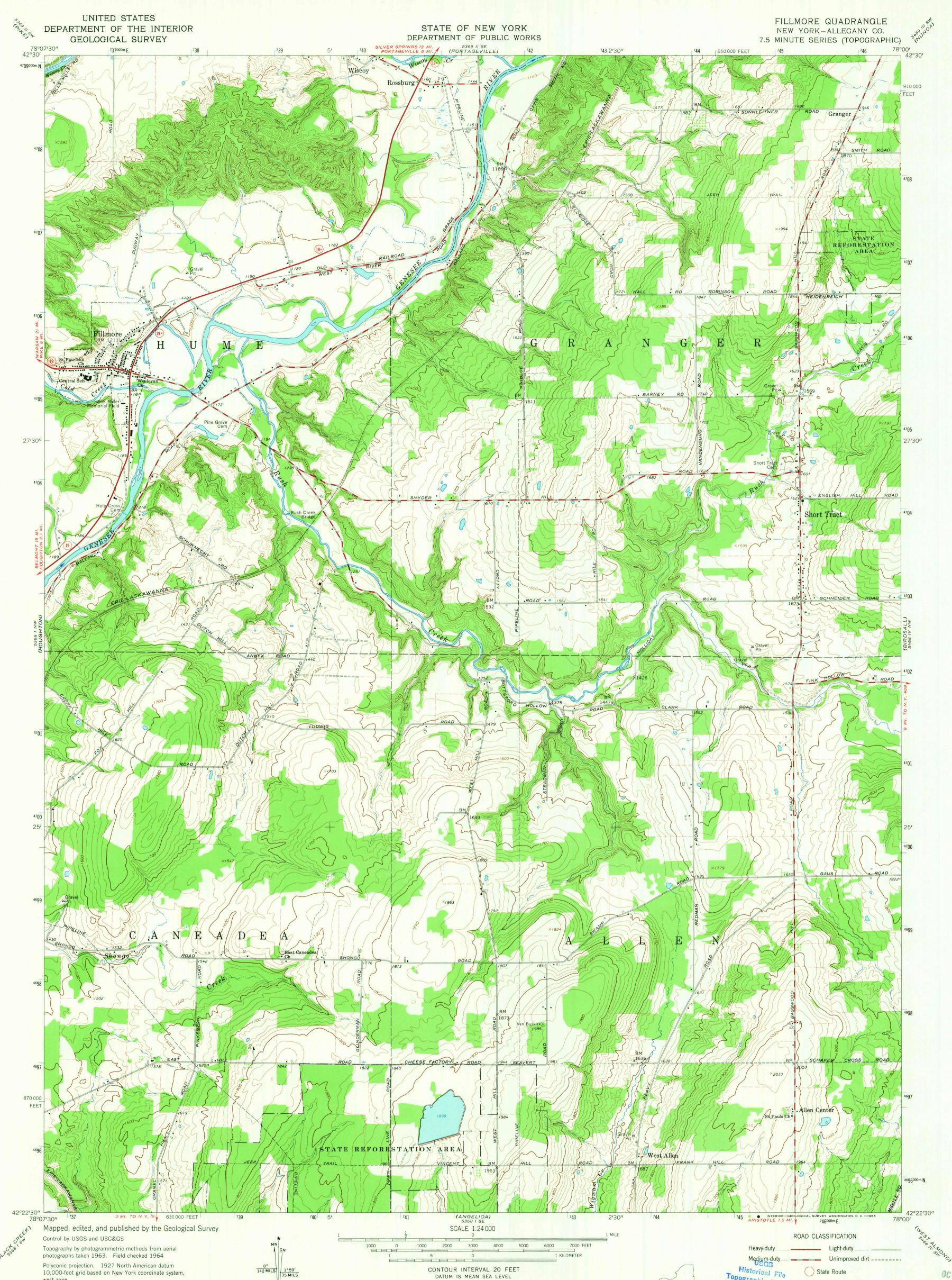
Polyconic projection. 1927 North American datum 10,000-foot grid based on New York coordinate system, west zone 1000-meter Universal Transverse Mercator grid ticks, zone 17, shown in blue
