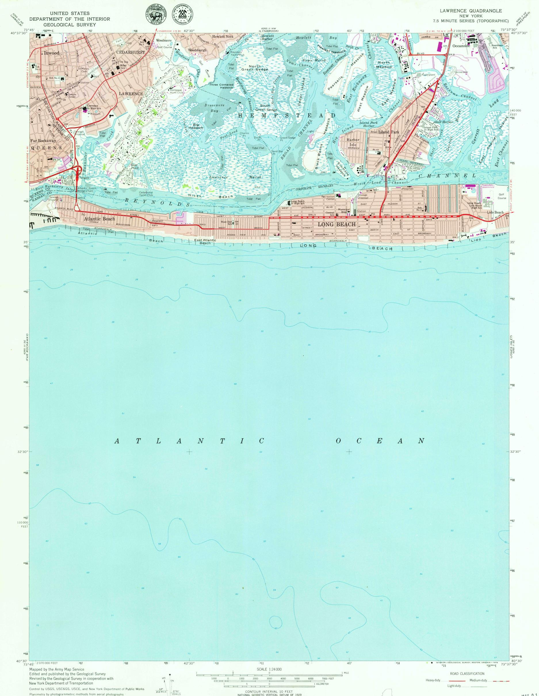
Planimetry by photogrammetric methods from aerial photographs taken 1941. Topography by planetable surveys 1943. Revised 1966
