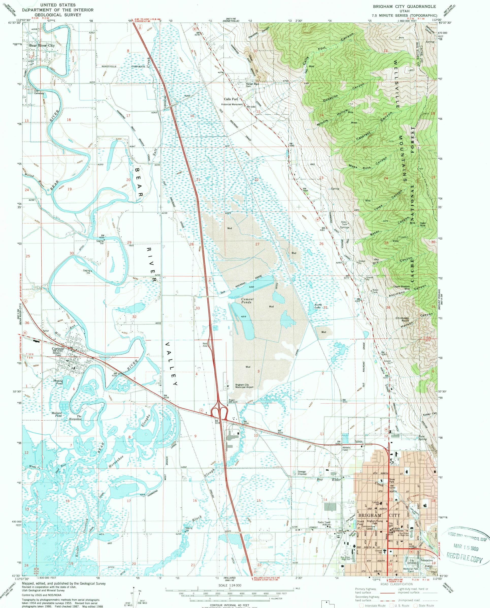
Projection and 10,000-foot grid ticks: Utah coordinate system, north zone (Lambert conformal conic) 1000-meter Universal Transverse Mercator grid, zone 12 1927 North American Datum To place on the predicted North American Datum 1983 move the projection lines 11 meters north and 66 meters east as shown by dashed corner ticks Fine red dashed lines indicate selected fence lines
