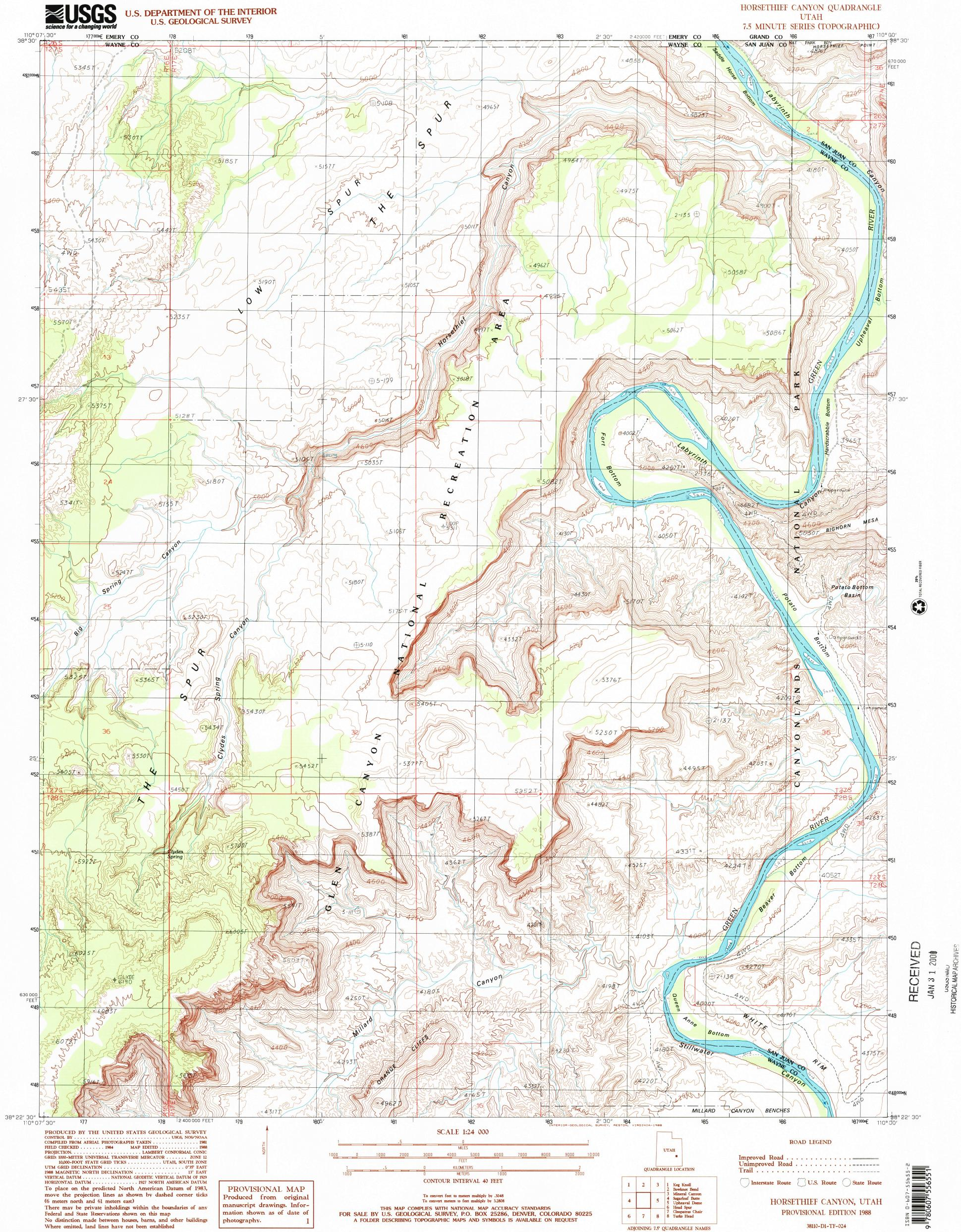
... NATIONAL GEODETIC VERTICAL DATUM OF 1929 HORIZONTAL DATUM ..... 1927 NORTH AMERICAN DATUM To place on the predicted North American Datum of 1983, move the projection lines as shown by dashed corner ticks (6 meters north and 61 meters east) There may be private inholdings within the boundaries of any Federal and State Reservations shown on this map No distinction made between houses, barns, and other buildings Where omitted, land lines have not been established
