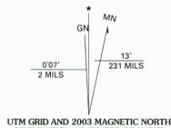
UTM GRID AND 2003 MAGNETIC NORTH DECLINATION AT CENTER OF SHEET
