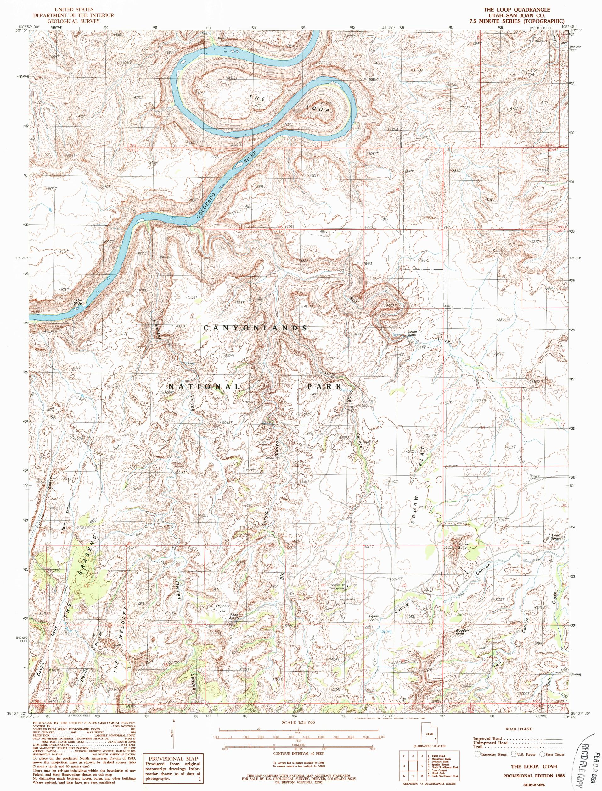
VERTICAL DATUM . . HORIZONTAL DATUM ..... 1927 NORTH AMERICAN DATUM To place on the predicted North American Datum of 1983, move the projection lines as shown by dashed corner ticks (5 meters north and 60 meters east) There may be private inholdings within the boundaries of any Federal and State Reservations shown on this map No distinction made between houses, barns, and other buildings Where omitted, land lines have not been established
