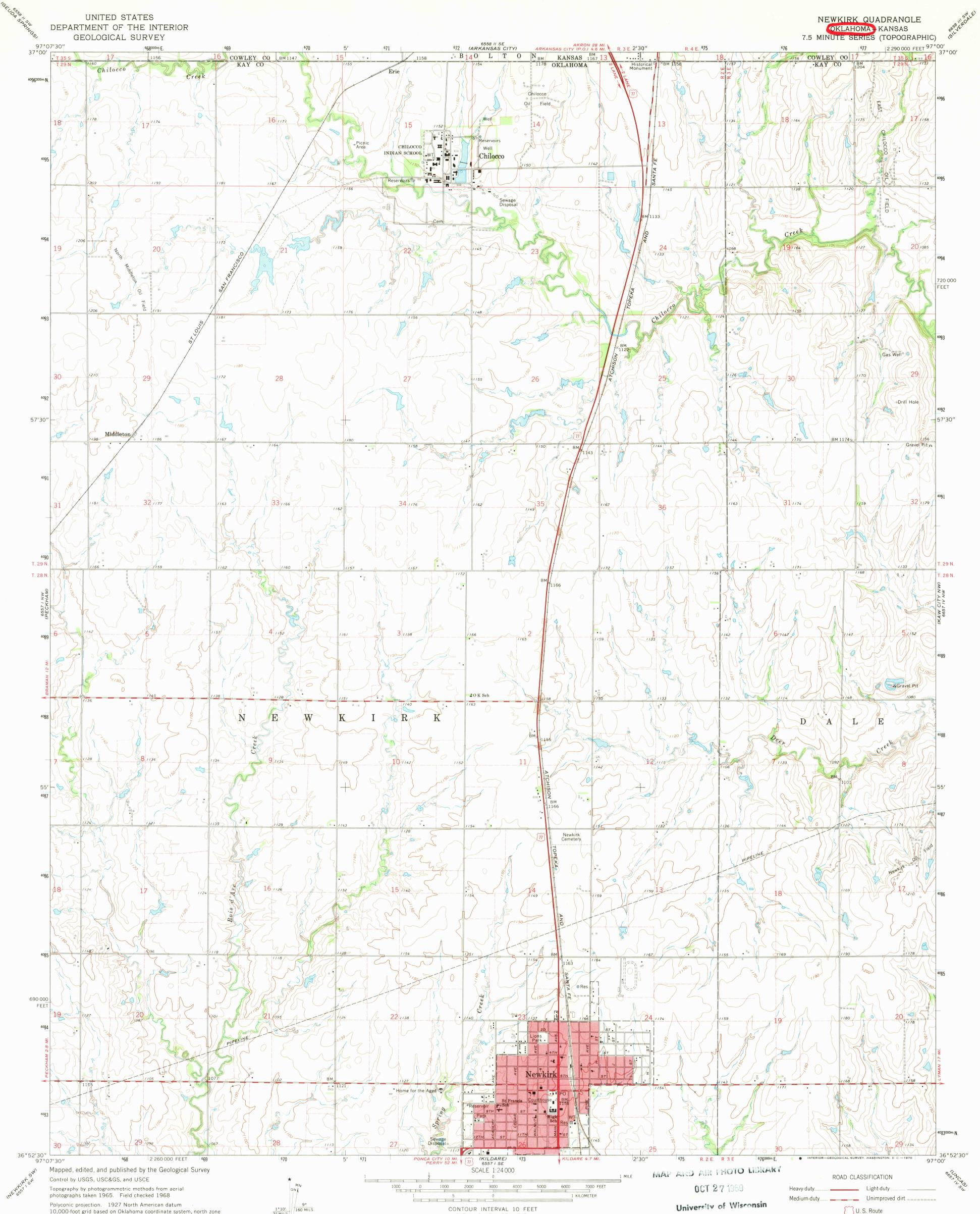
Polyconic projection. 1927 North American datum 10,000-foot grid based on Oklahoma coordinate system, north zone 1000-meter Universal Transverse Mercator grid ticks, zone 14, shown in blue
