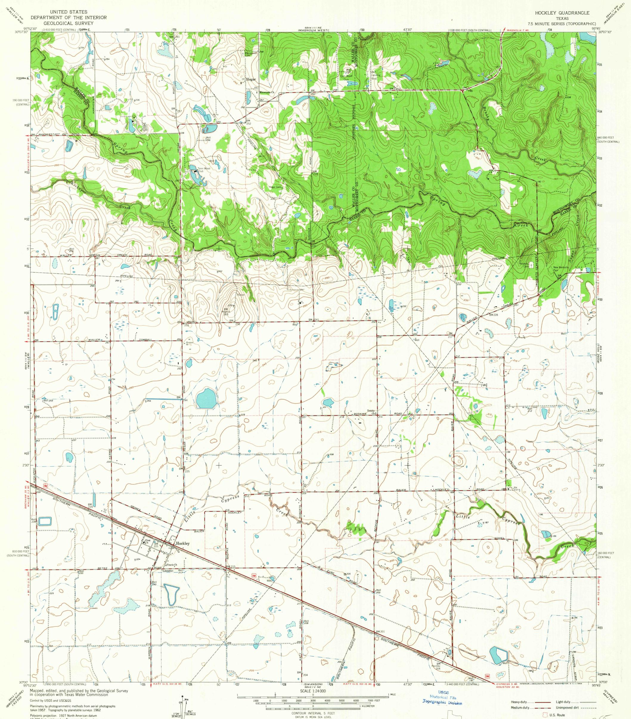
Polyconic projection. 1927 North American datum 10,000-foot grid based on Texas coordinate system, south central and central zones 1000-meter Universal Transverse Mercator grid ticks, zone 15, shown in blue
