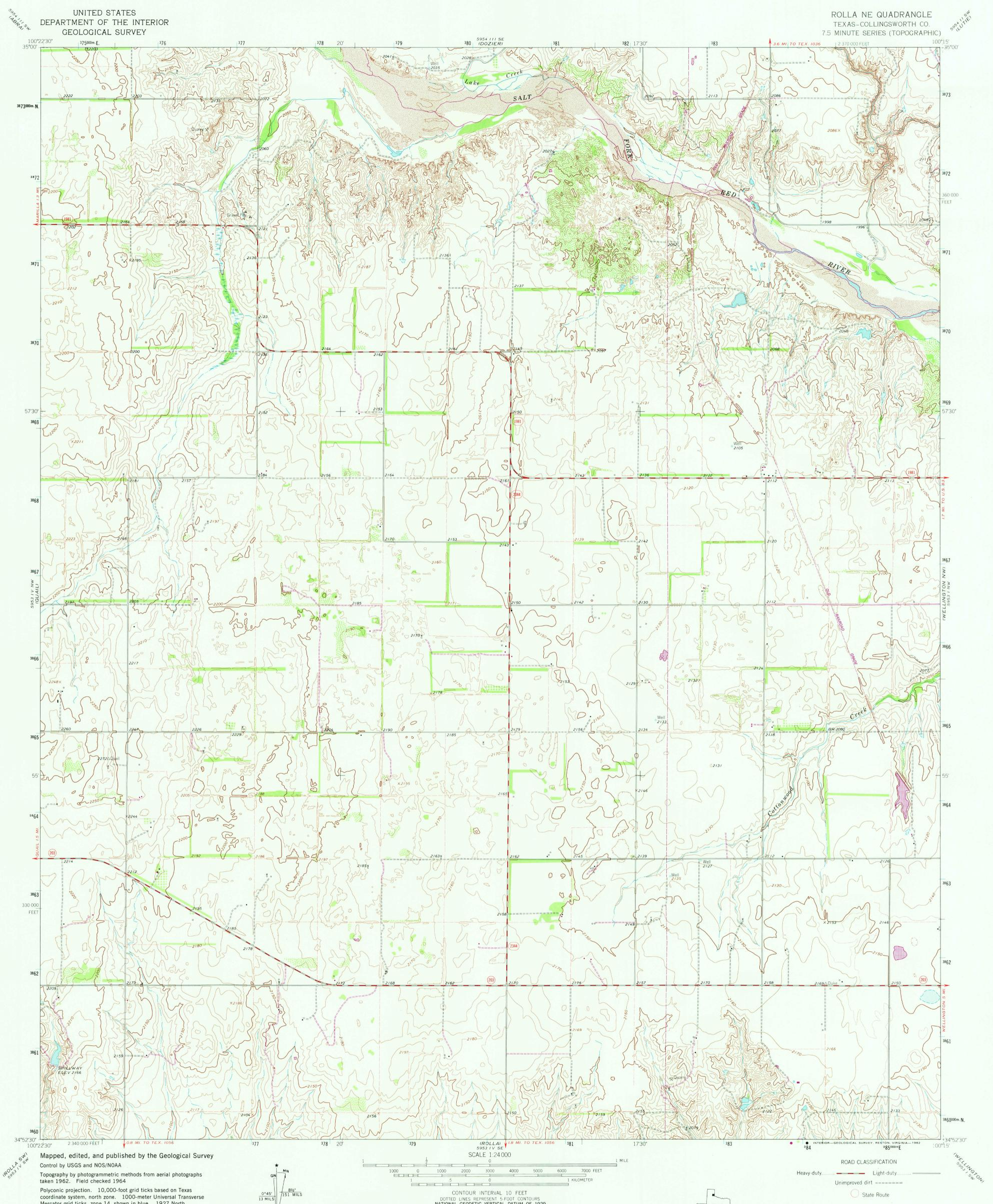
Polyconic projection. 10,000-foot grid ticks based on Texas coordinate system, north zone. 1000-meter Universal Transverse Mercator grid ticks, zone 14, shown in blue. 1927 North American Datum. To place on the predicted North American Datum 1983 move the projection lines 2 meters south and 36 meters east as shown by dashed corner ticks
