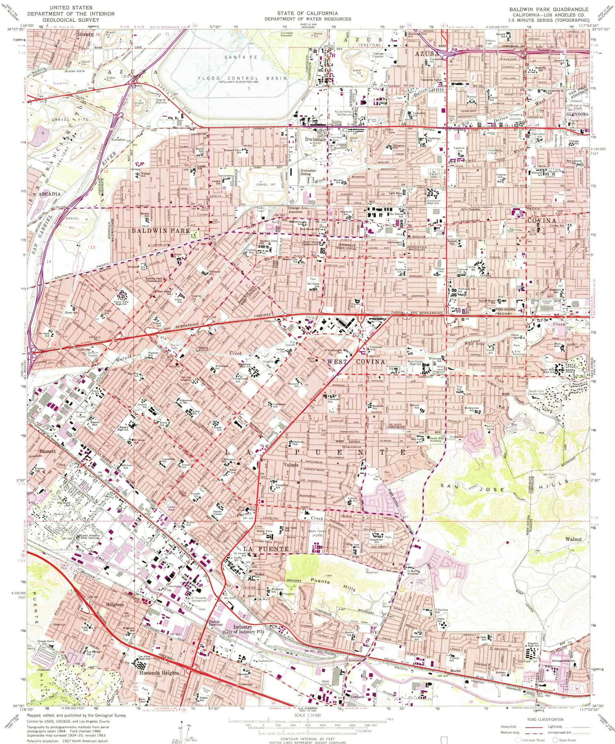
Polyconic projection. 1927 North American datum 10,000-foot grid based on California coordinate system, zone 7 1000-meter Universal Transverse Mercator grid ticks, zone 11, shown in blue
