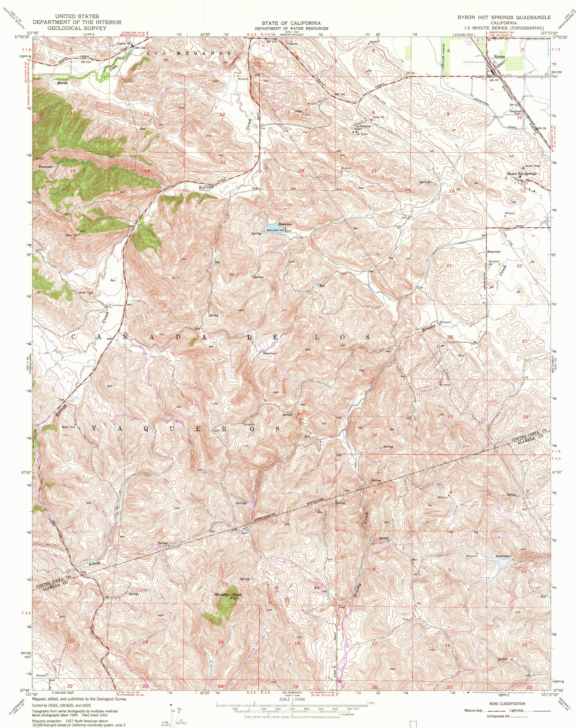
Polyconic projection. 1927 North American datum 10,000-foot grid based on California coordinate system, zone 3 1000-metre Universal Transverse Mercator grid ticks, zone 10, shown in blue
