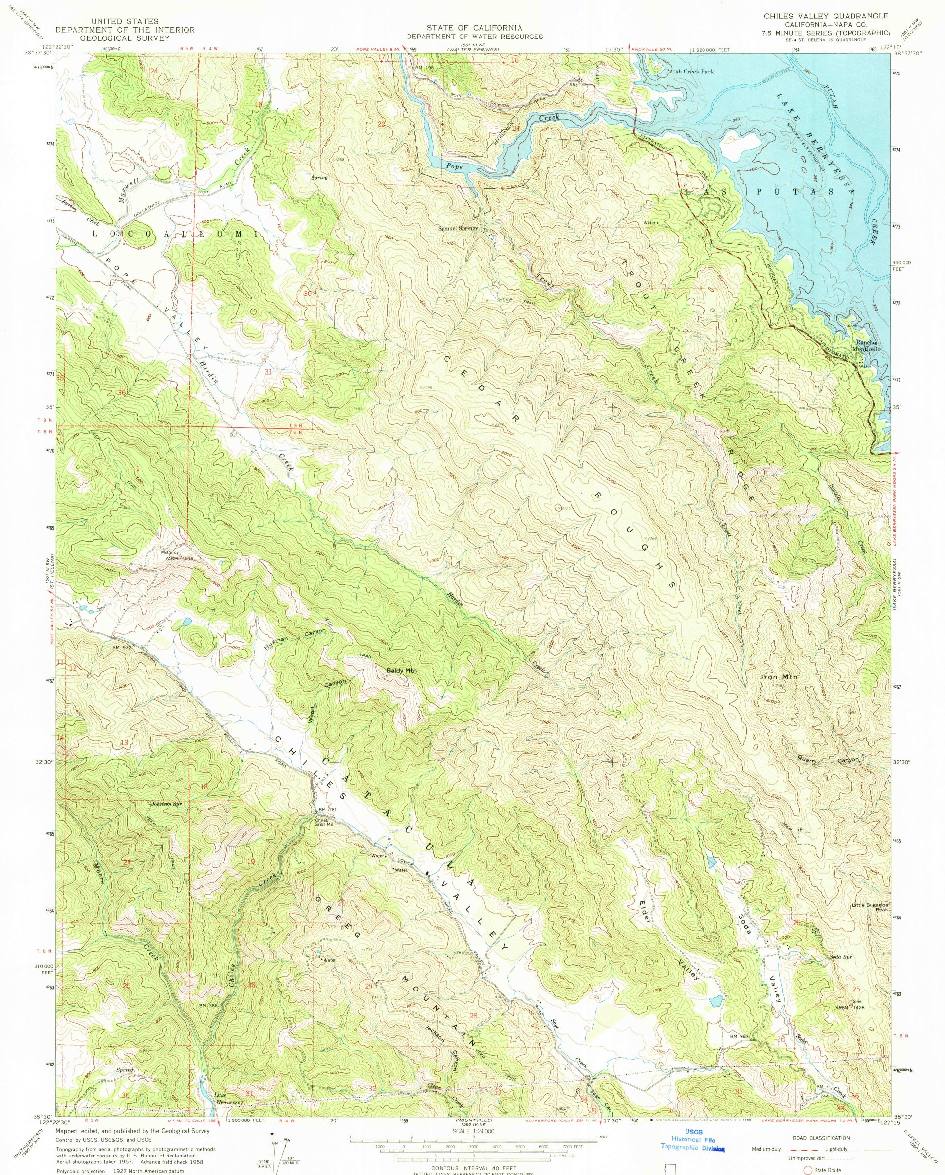
Polyconic projection. 1927 North American datum 10,000-foot grid based on California coordinate system, zone 2 1000-meter Universal Transverse Mercator grid ticks, zone 10, shown in blue
