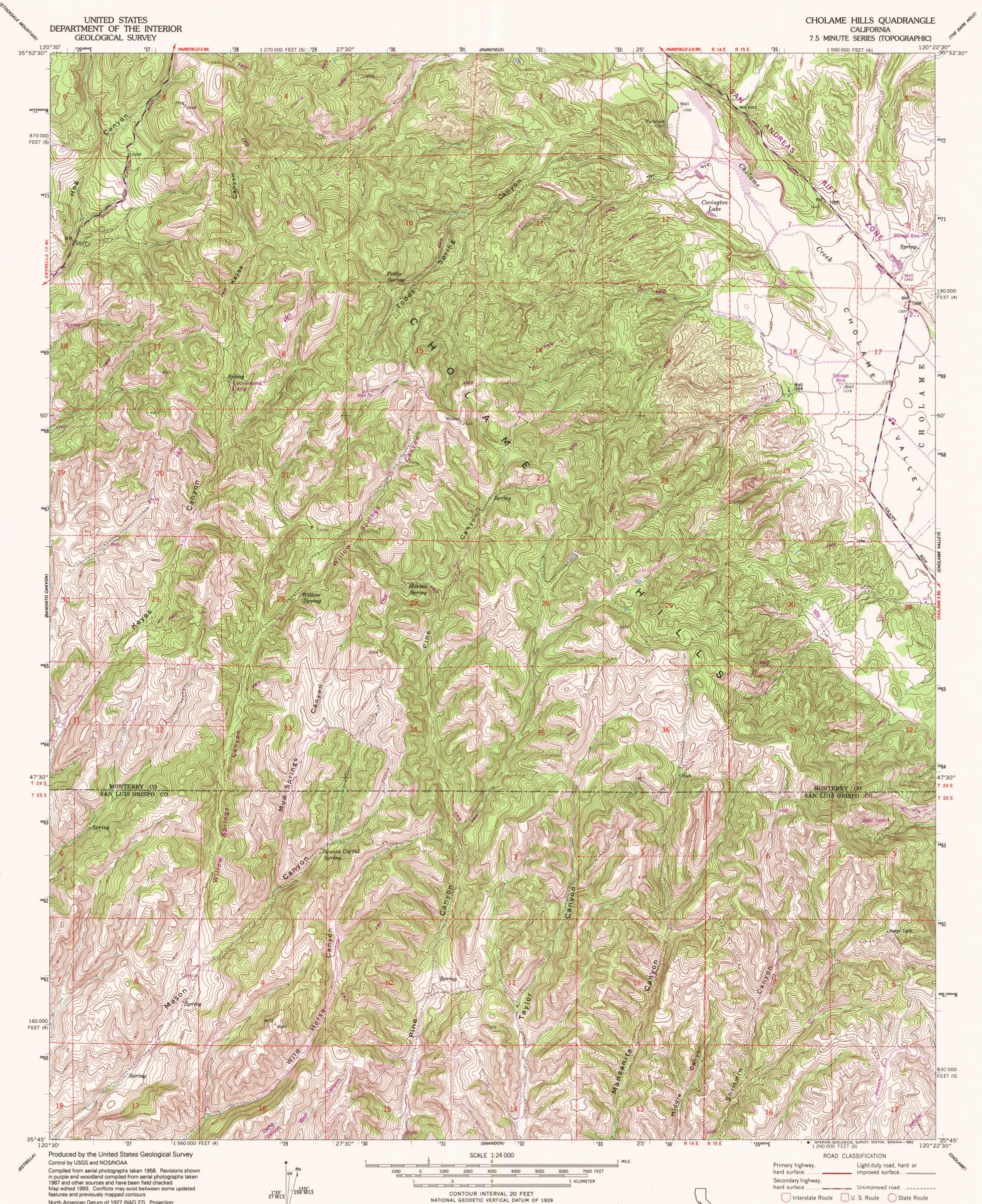
North American Datum of 1927 (NAD 27). Projection: California Coordinate System, zone 4 (Lambert Conformal Conic) 10 000-foot grid ticks: California Coordinate System, zones 4 and 5 Blue 1000-meter Universal Transverse Mercator grid ticks, zone 10 North American Datum 1983 (NAD 83) is shown by dashed corner ticks. The values of the shift between NAD 27 and NAD 83 for 7.5 minute intersections is given in USGS Bulletin 1875
