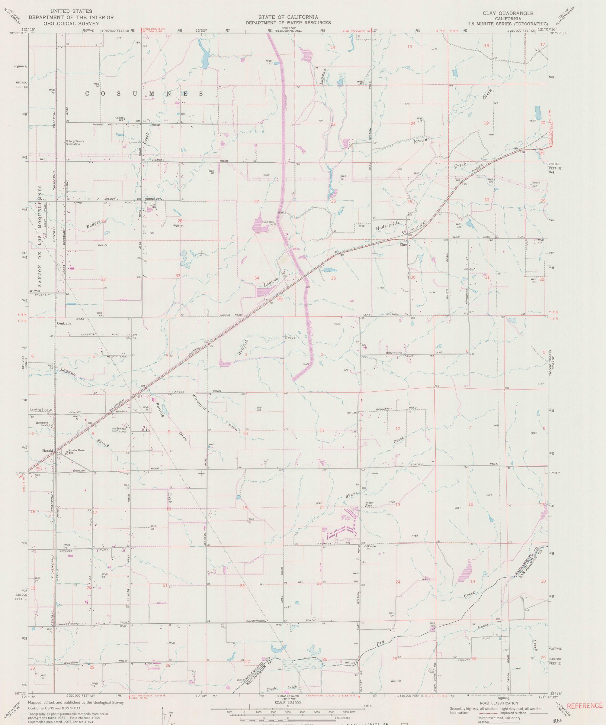
Supersedes map dated 1907, revised 1953 Polyconic projection. 1927 North American datum 10,000-foot grids based on California coordinate system, zones 2 and 3 1000-meter Universal Transverse Mercator grid ticks, zone 10, shown in blue To place on the predicted North American Datum 1983 move the projection lines 14 meters north and 92 meters east as shown by dashed corner ticks
