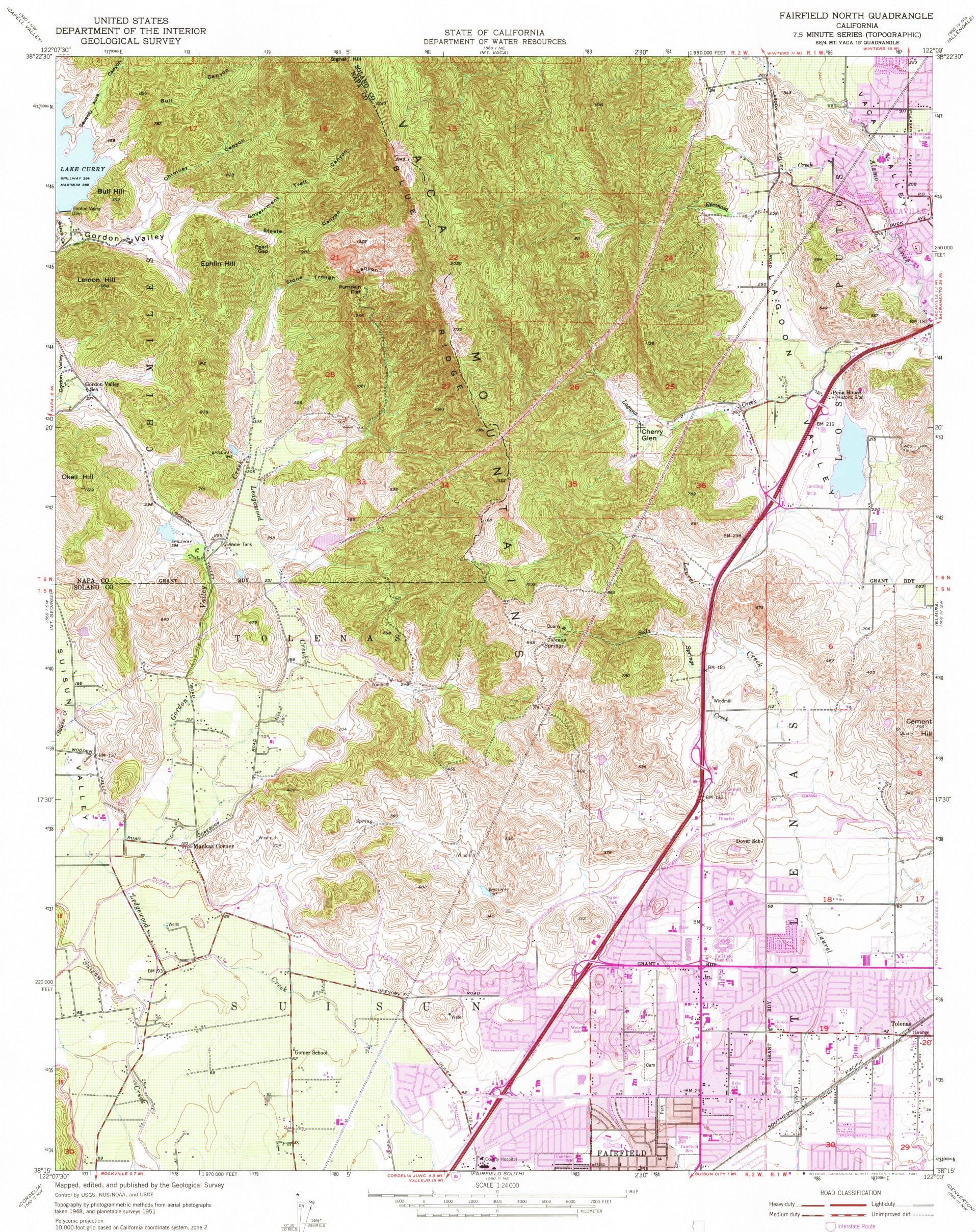
10,000-foot grid based on California coordinate system, zone 2 1000-meter Universal Transverse Mercator grid ticks, zone 10 shown in blue. 1927 North American Datum To place on the predicted North American Datum 1983 move the projection lines 15 meters north and 94 meters east as shown by dashed corner ticks Red tint indicates area in which only
