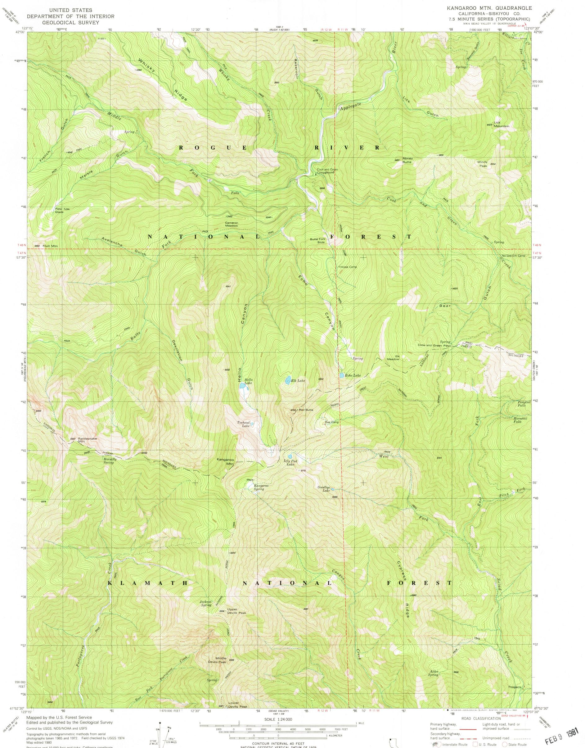
Projection and 10,000-foot grid ticks: California coordinate system, zone 1 (Lambert conformal conic) 1000-meter Universal Transverse Mercator grid, zone 10 1927 North American Datum To place on the predicted North American Datum 1983 move the projection lines 20 meters north and 95 meters east as shown by dashed corner ticks Certain land lines are omitted because of insufficient data There may be private inholdings within the boundaries of
