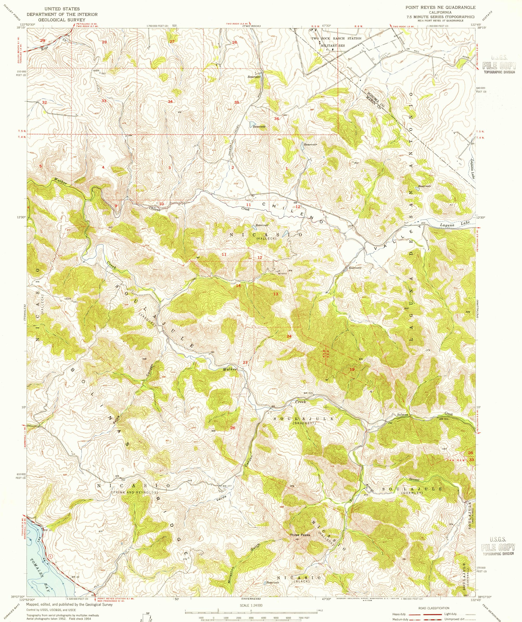
Polyconic projection. 1927 North American datum 10,000-foot grids based on California coordinate system, zones 2 and 3 Hydrography compiled from USC&GS Chart 5603 Dashed land lines indicate approximate locations Unchecked elevations are shown in brown
