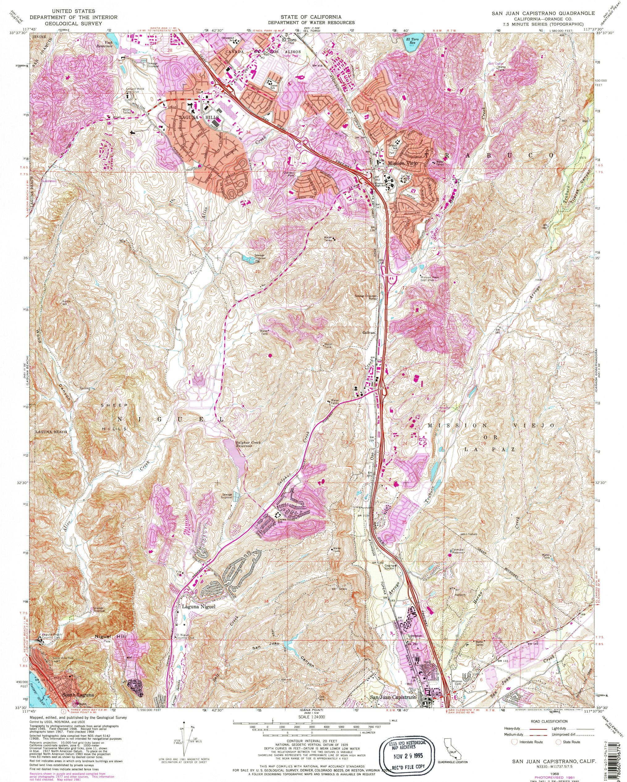
Polyconic projection. 10,000-foot grid ticks based on California coordinate system, zone 6. 1000-meter Universal Transverse Mercator grid ticks, zone 11, shown in blue. 1927 North American Datum. To place on the predicted North American Datum 1983 move the projection lines 83 meters east as shown by dashed corner ticks Red tint indicates areas in which only landmark buildings are shown Dotted land lines established by private surveys Fine red dashed lines indicate selected fence lines
