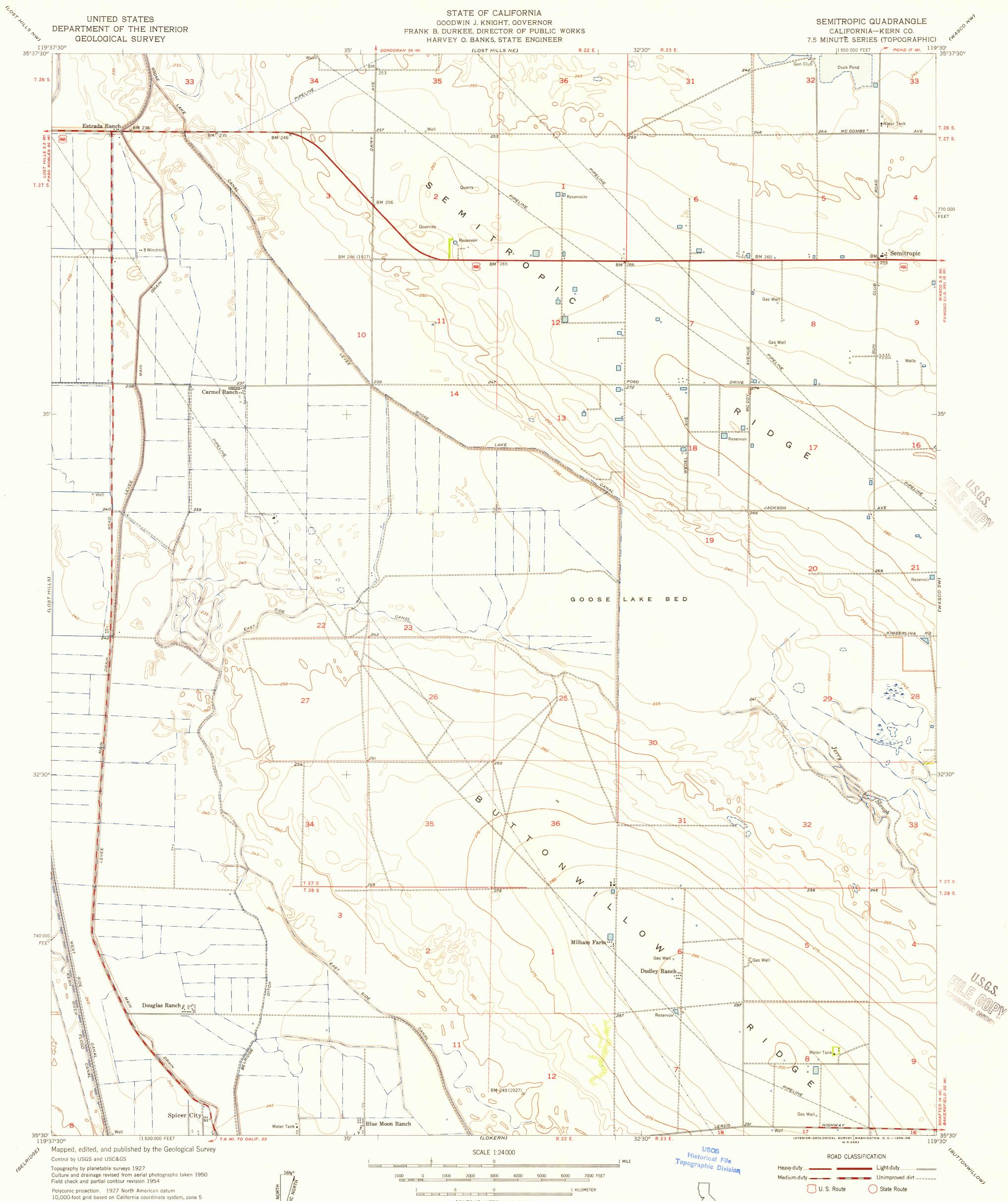
Polyconic projection. 1927 North American datum 10,000-foot grid based on California coordinate system, zone 5 Dashed land lines indicate approximate locations The northeast portion of this map lies within a subsidence area Contouring not corrected to later vertical control adjustments All vertical control established 1954 unless otherwise noted
