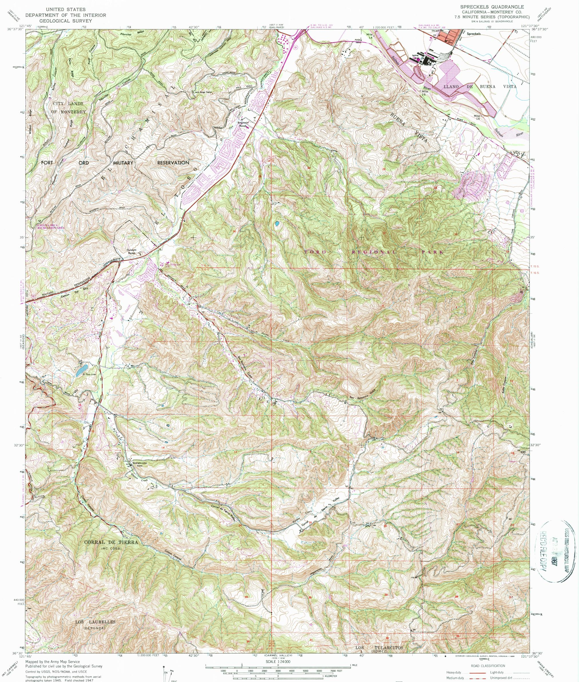
Polyconic projection. 1927 North American datum 10,000-foot grid based on California coordinate system, zone 4 1000-meter Universal Transverse Mercator grid ticks, zone 10, shown in blue To place on the predicted North American Datum 1983 move the projection lines 11 meters north and 93 meters east as shown by dashed corner ticks
