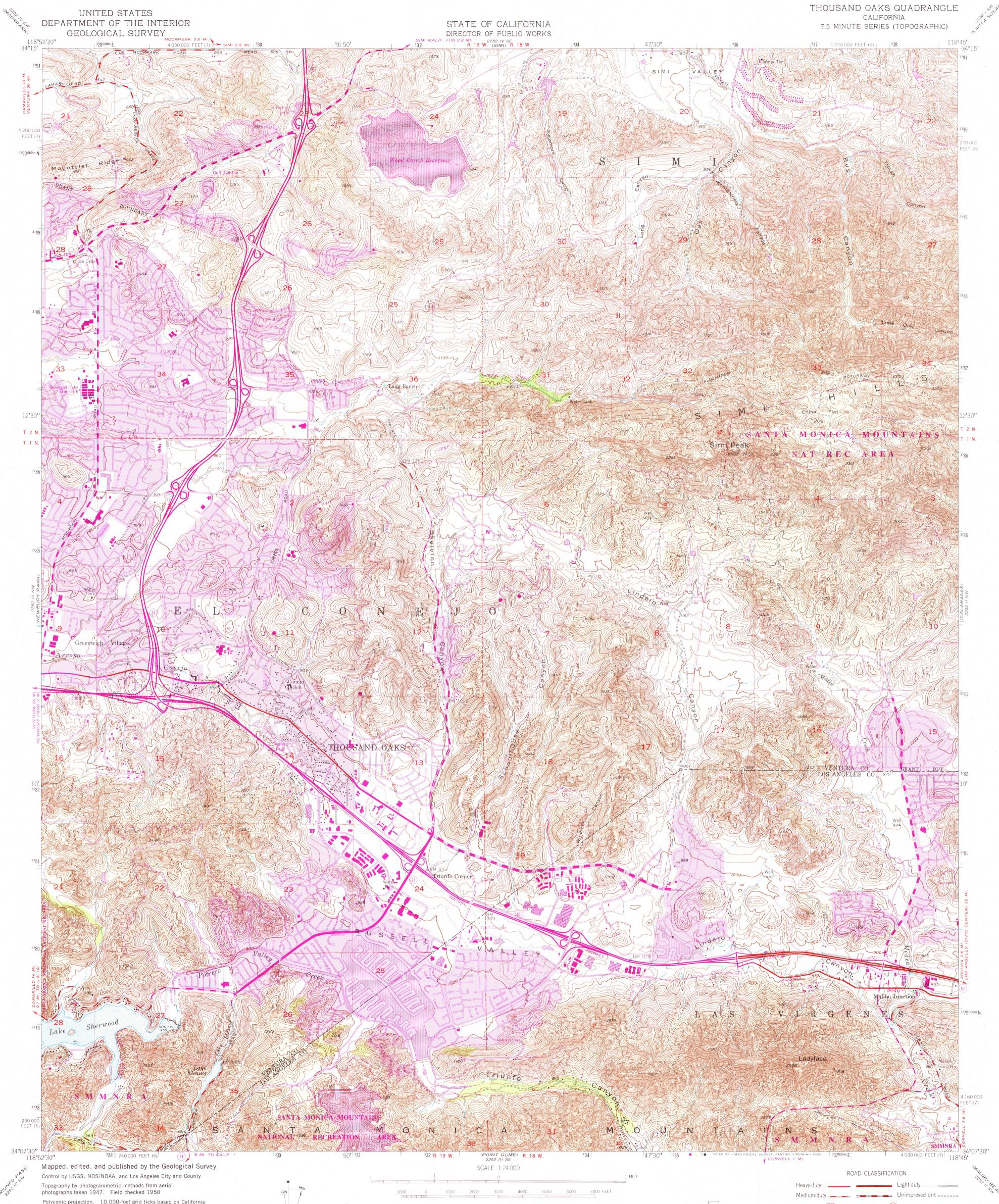
coordinate system, zones 5 and 7. 1000-meter Universal Transverse Mercator grid ticks, zone 11 shown in blue 1927 North American Datum. To place on the predicted North American Datum 1983 move the projection lines 3 meters north and 85 meters east as shown by dashed corner ticks Section lines within land grants were established by private survey There may be private inholdings within the boundaries of the National or State reservations shown on this map
