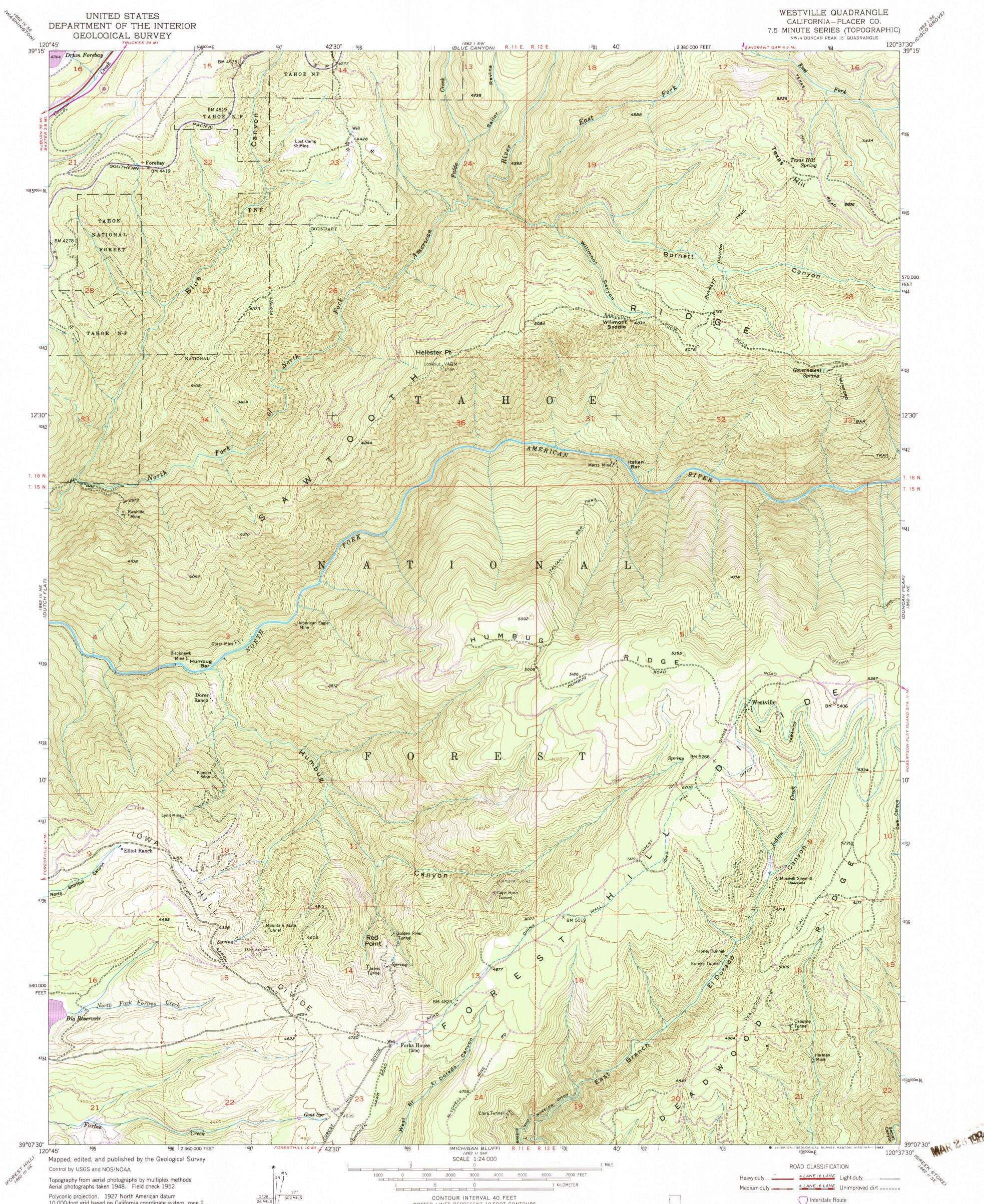
10,000-foot grid based on California coordinate system, zone 2 1000-meter Universal Transverse Mercator grid ticks, zone 10, shown in blue To place on the predicted North American Datum 1983 move the projection lines 15 meters north and 89 meters east as shown by dashed corner ticks
