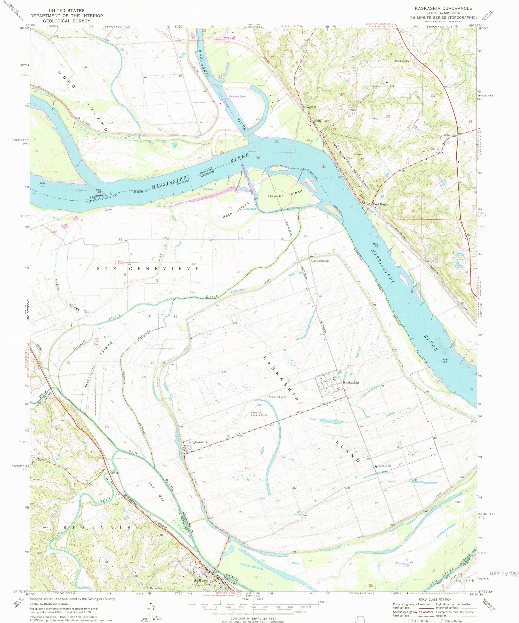
Polyconic projection. 1927 North American datum 10,000-foot grids based on Illinois coordinate system, west zone and Missouri coordinate system, east zone 1000-meter Universal Transverse Mercator grid ticks, zone 16, shown in blue
