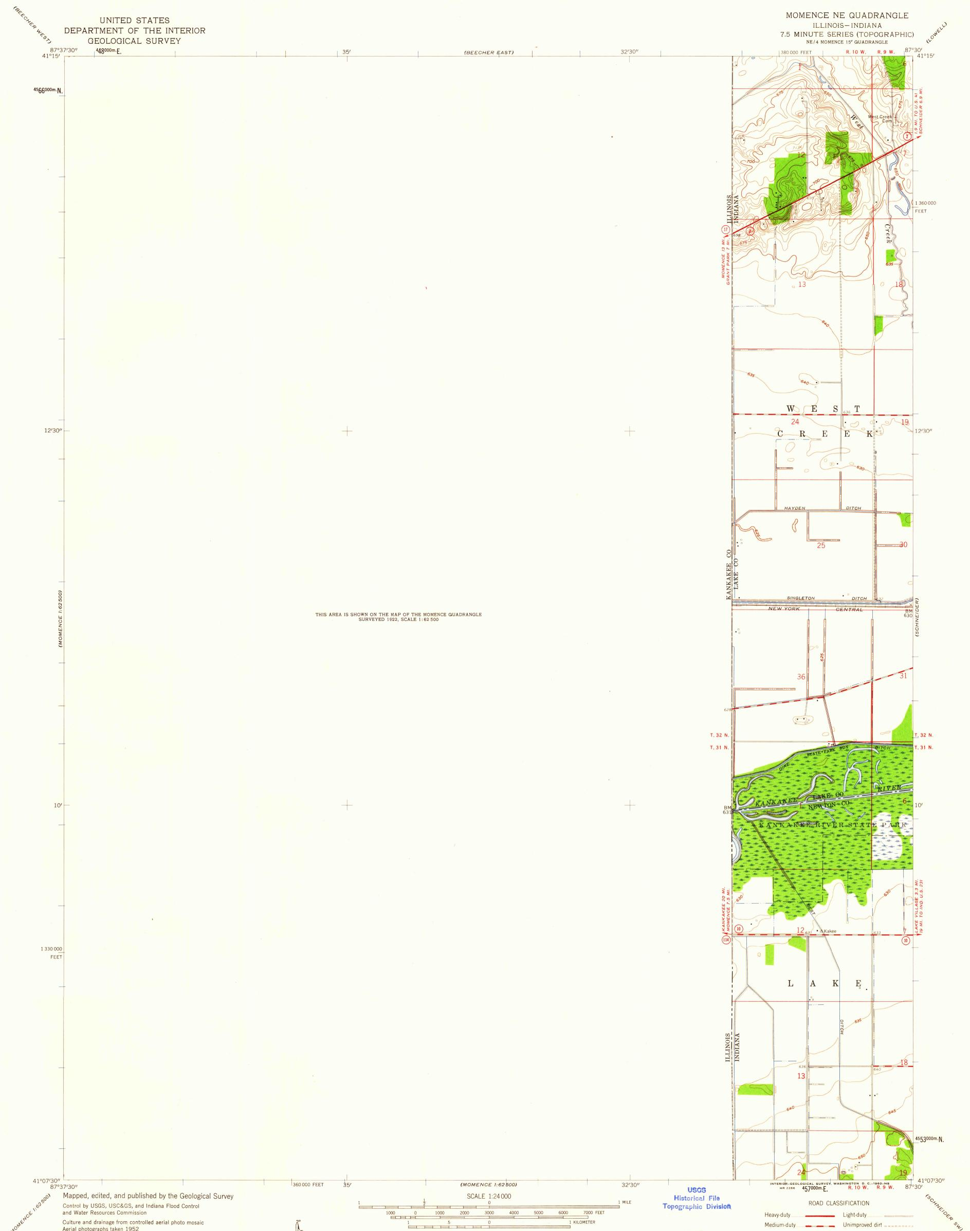
Aerial photographs taken 1952 Topography by planetable surveys 1959 Polyconic projection. 1927 North American datum 10,000-foot grid based on Indiana coordinate system, west zone 1000-meter Universal Transverse Mercator grid ticks, zone 16, shown in blue
