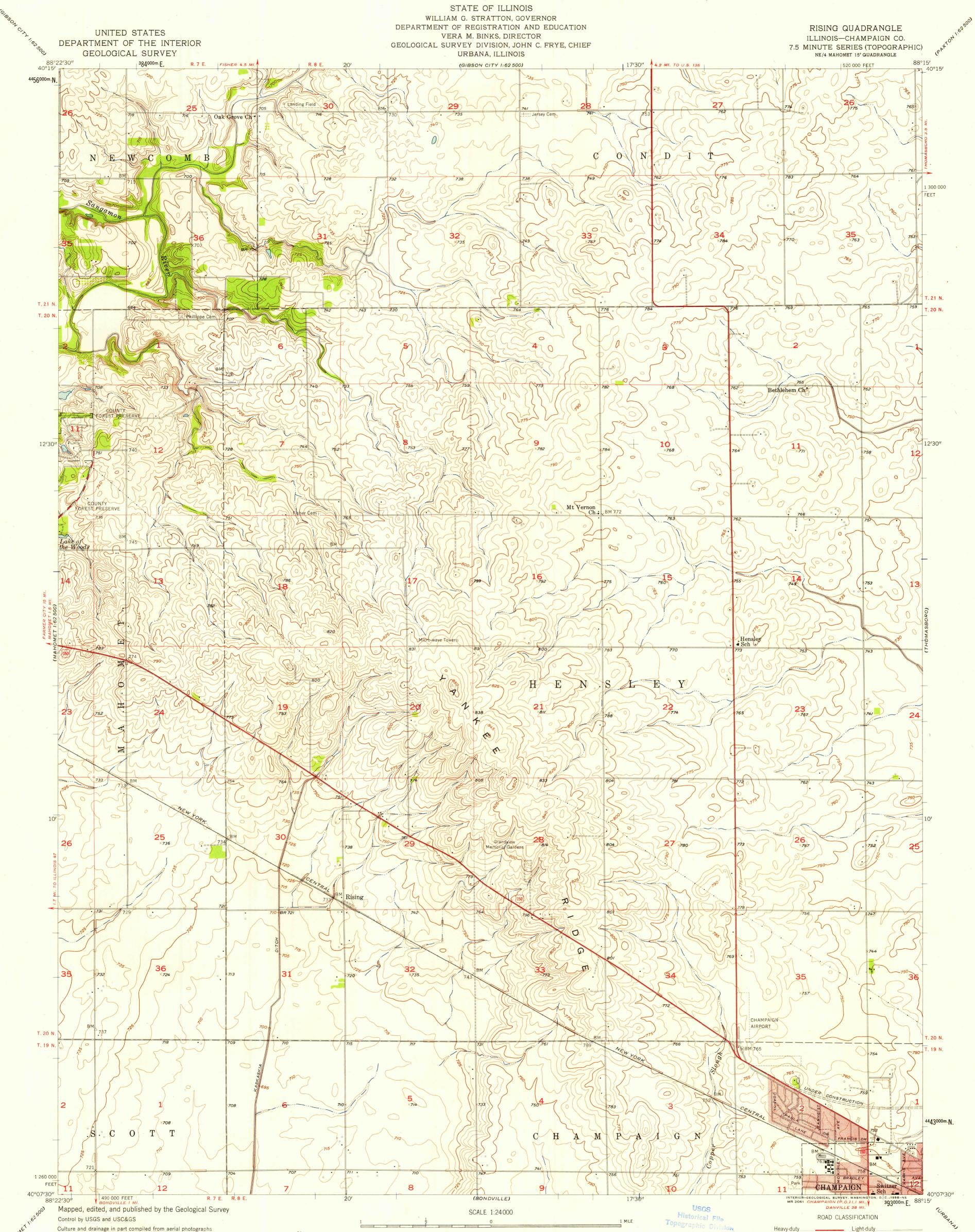
taken 1954. Topography by planetable surveys 1949–1950 and 1957 Polyconic projection. 1927 North American datum 10,000-foot grid based on Illinois coordinate system, east zone 1000-meter Universal Transverse Mercator grid ticks, zone 16, shown in blue Red tint indicates area in which only landmark buildings are shown
