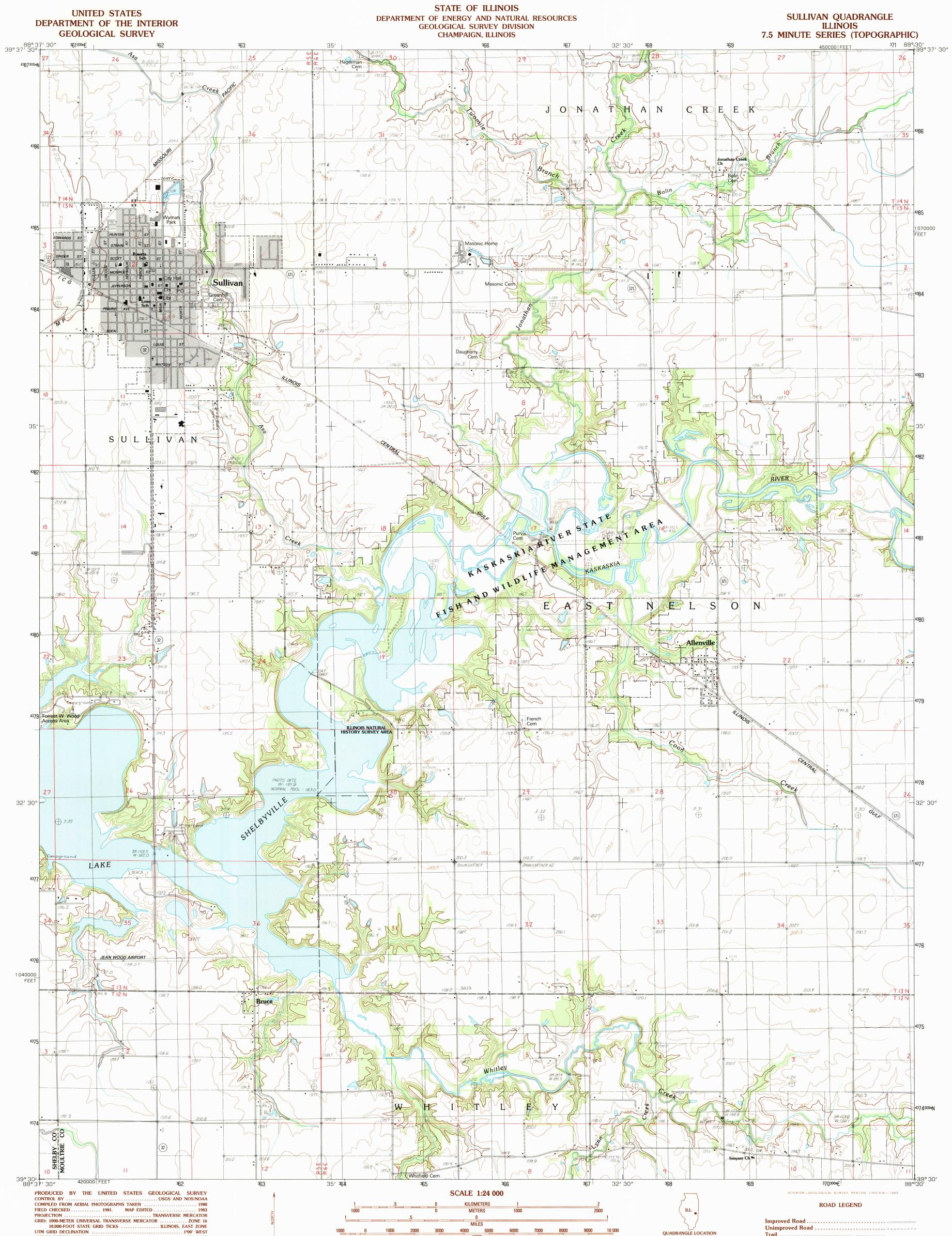
. 1°00' WEST 1983 MAGNETIC NORTH DECLINATION ... . 1°00' EAST VERTICAL DATUM ..... NATIONAL GEODETIC VERTICAL DATUM OF 1929 HORIZONTAL DATUM .... ..... 1927 NORTH AMERICAN DATUM To place on the predicted North American Datum of 1983 move the projection lines as shown by dashed corner ticks (1 meter south and 5 meters east) There may be private inholdings within the boundaries of any Federal and State reservations shown on this map Gray tint indicates area in which selected buildings are shown
