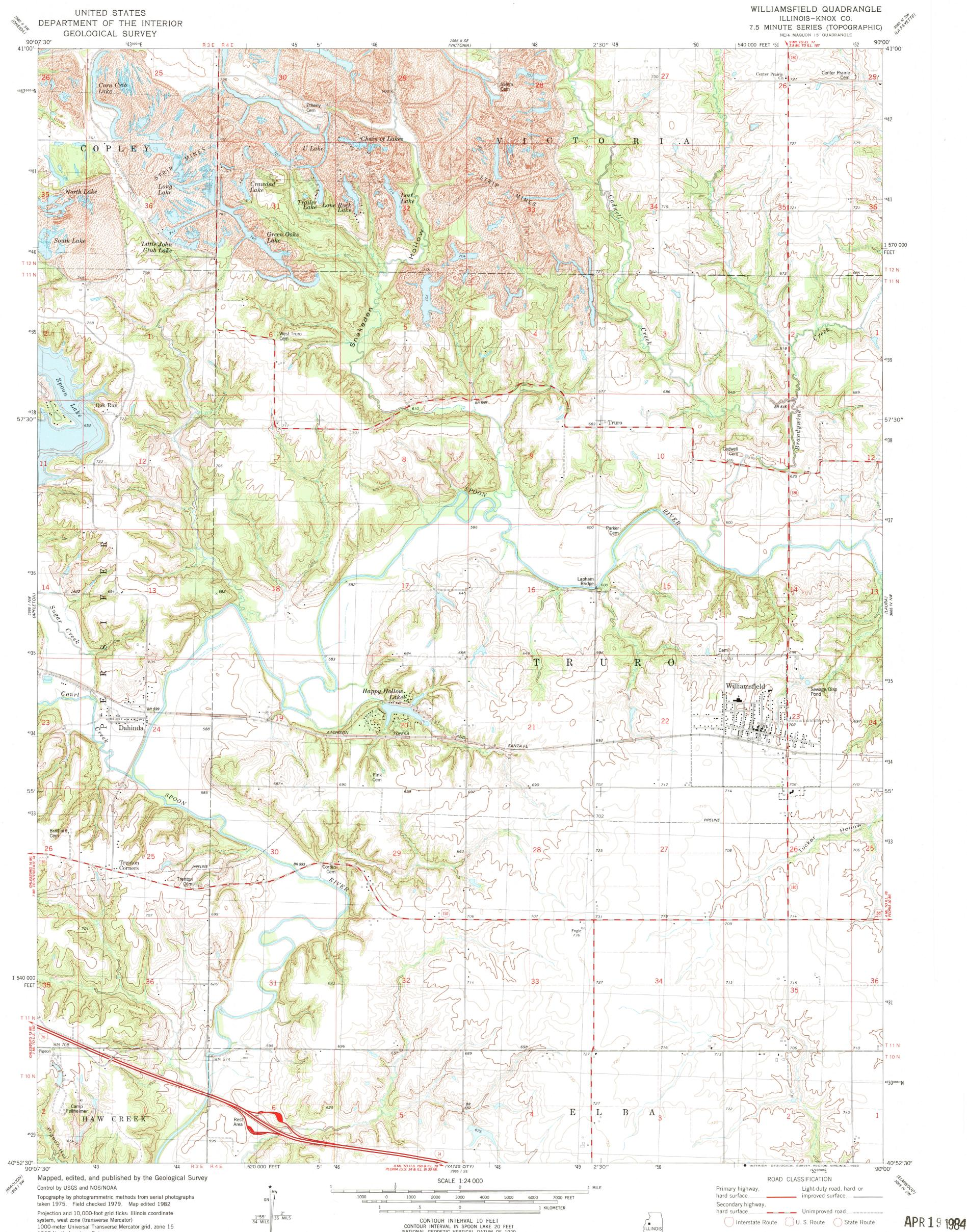
system, west zone (transverse Mercator) 1000-meter Universal Transverse Mercator grid, zone 15 1927 North American Datum To place on the predicted North American Datum 1983 move the projection lines 1 meter north and 9 meters east as shown by dashed corner ticks Fine red dashed lines indicate selected fence and field lines where
