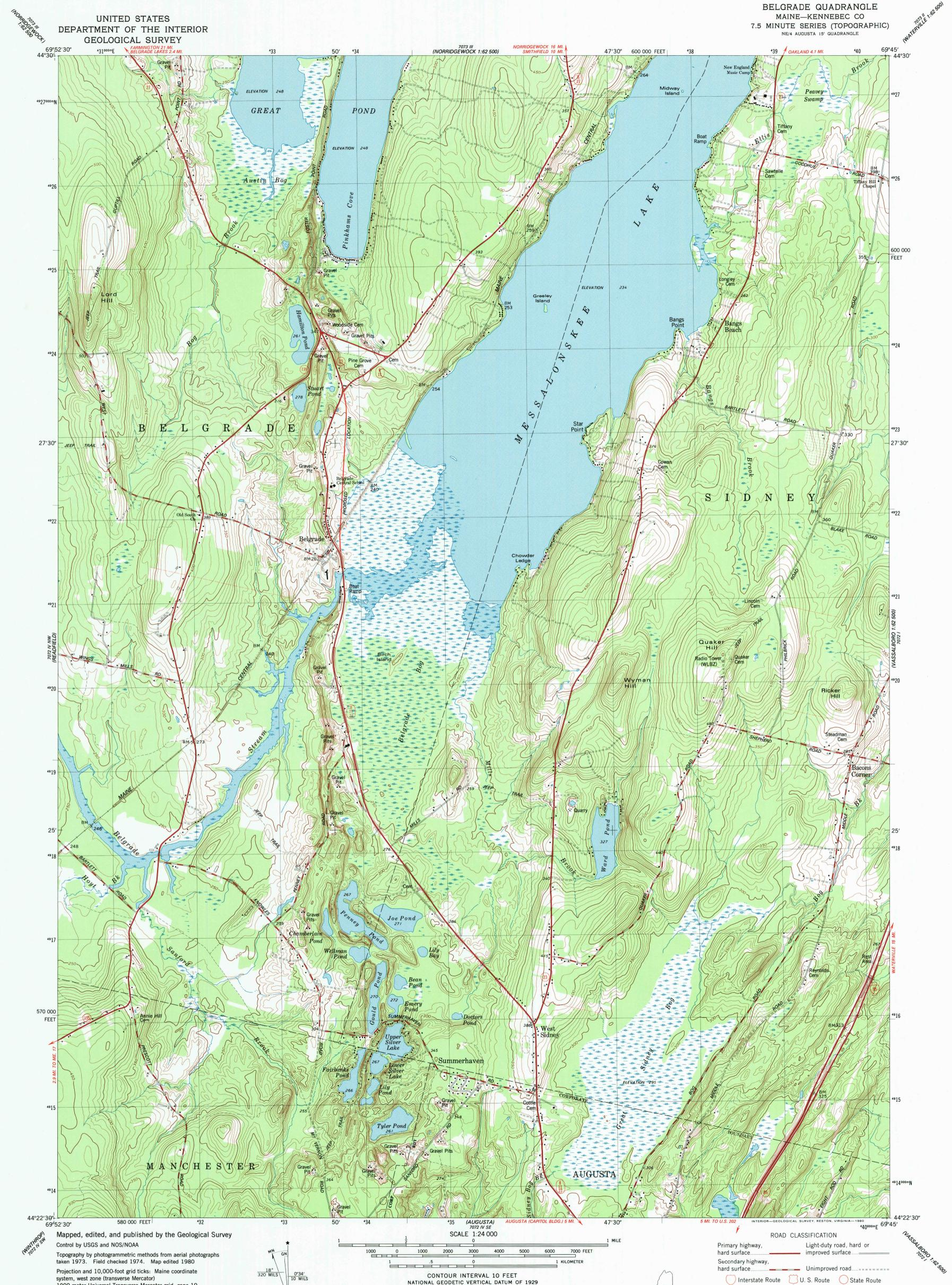
system, west zone (transverse Mercator) 1000-meter Universal Transverse Mercator grid, zone 19 1927 North American Datum To place on the predicted North American Datum 1983 move the projection lines 3 meters south and 42 meters west as shown by dashed corner ticks
