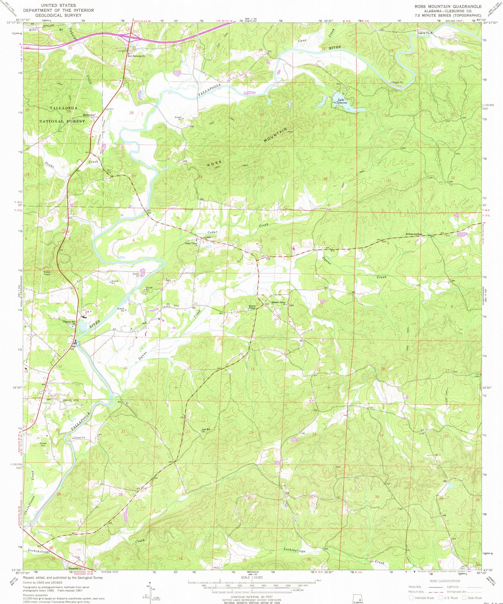
1000-meter Universal Transverse Mercator grid ticks, zone 16, shown in blue. 1927 North American Datum To place on the predicted North American Datum 1983 move the projection lines 10 meters south and 5 meters west as shown by dashed corner ticks
