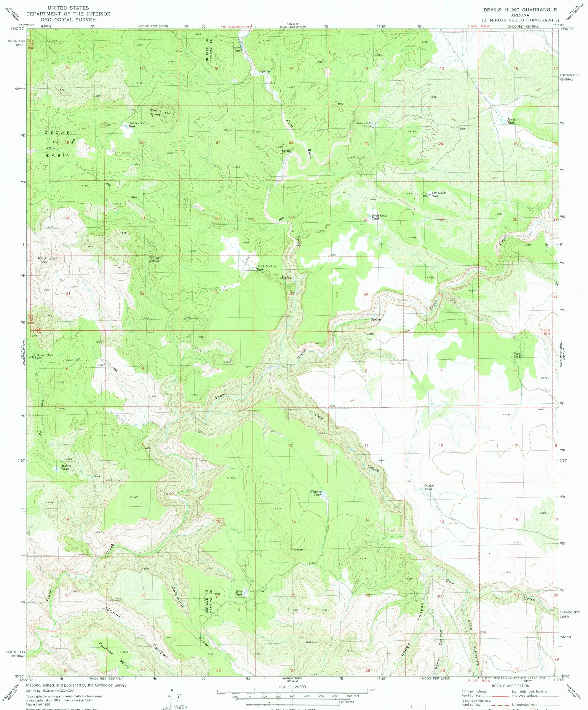
Projection: Arizona coordinate system, central zone (transverse Mercator) 10,000-foot grid ticks based on Arizona coordinate system, central and west zones 1000-meter Universal Transverse Mercator grid, zone 12 1927 North American Datum To place on the predicted North American Datum 1983 move the projection lines 2 meters north and 69 meters east as shown by dashed corner ticks
