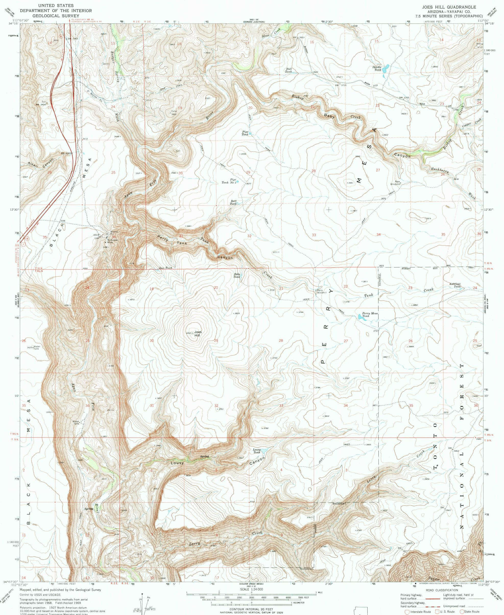
1000-meter Universal Transverse Mercator grid ticks, zone 12, shown in blue To place on the predicted North American Datum 1983, move the projection lines 1 meter south and 66 meters east as shown by dashed corner ticks
