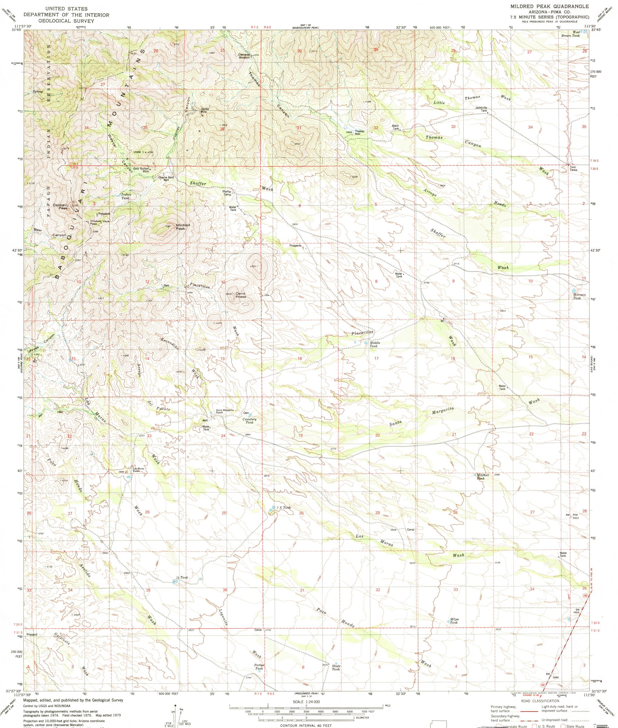
system, central zone (transverse Mercator) 1000-meter Universal Transverse Mercator grid, zone 12 1927 North American datum To place on the predicted North American Datum 1983, move the projection lines 8 meters south and 64 meters east as shown by dashed corner ticks
