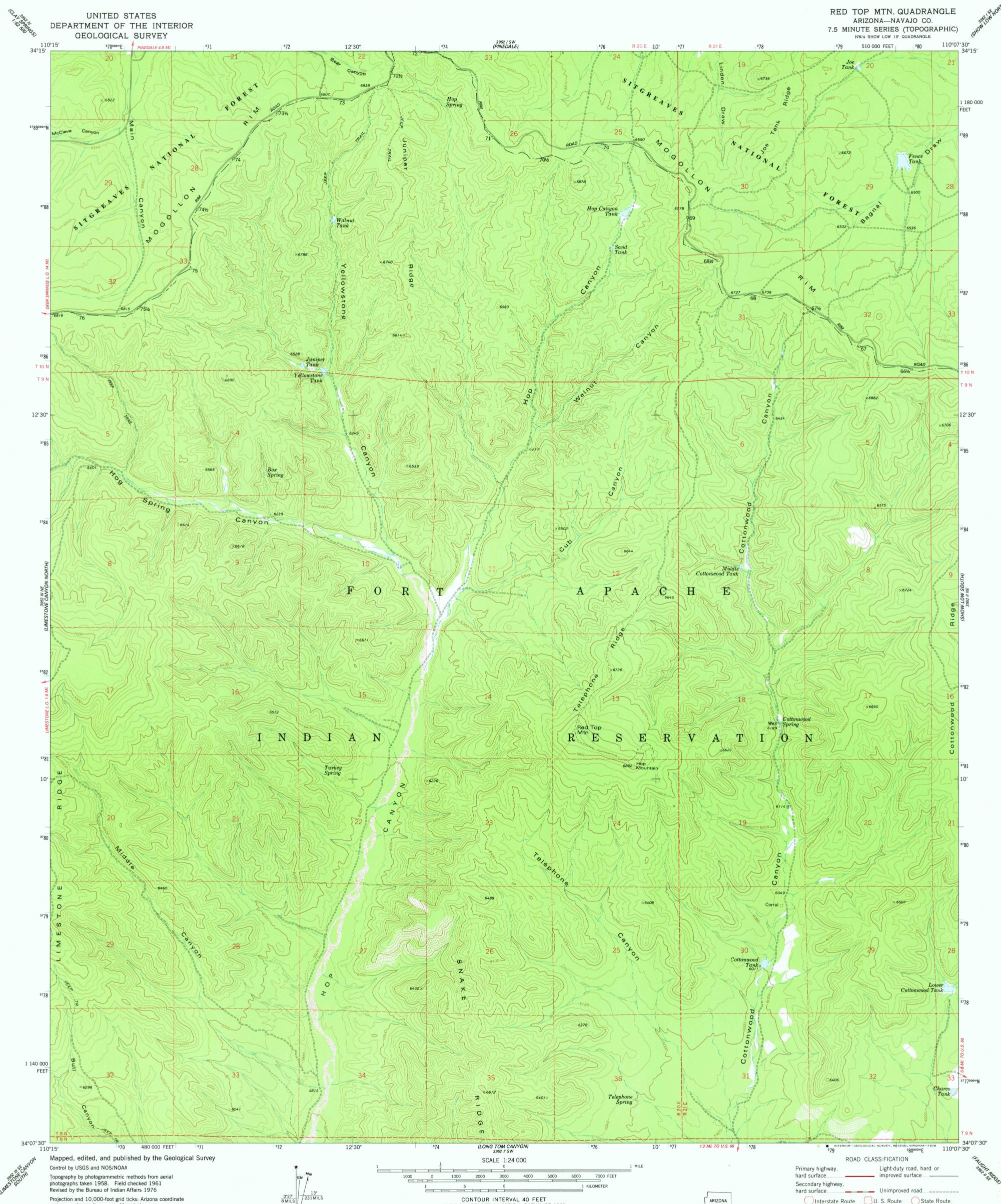
Projection and 10,000-foot grid ticks: Arizona coordinate system, east zone (transverse Mercator) 1000-meter Universal Transverse Mercator grid ticks, zone 12, shown in blue. 1927 North American datum Fine red dashed lines indicate selected fence lines Where omitted, land lines have not been established
