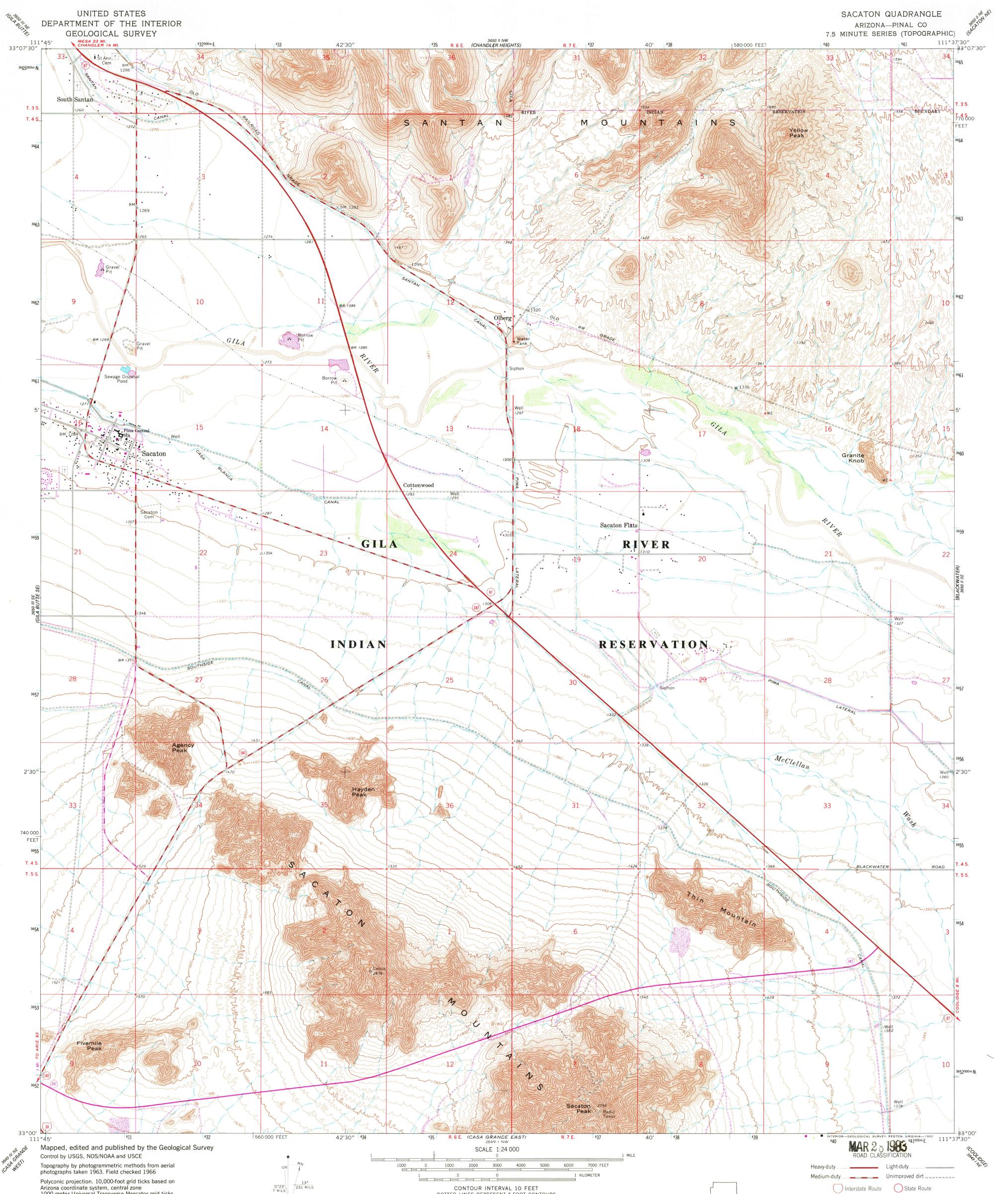
Arizona coordinate system, central zone 1000-meter Universal Transverse Mercator grid ticks, zone 12, shown in blue. 1927 North American Datum To place on the predicted North American Datum 1983 move the projection lines 2 meters south and 64 meters east as shown by dashed corner ticks
