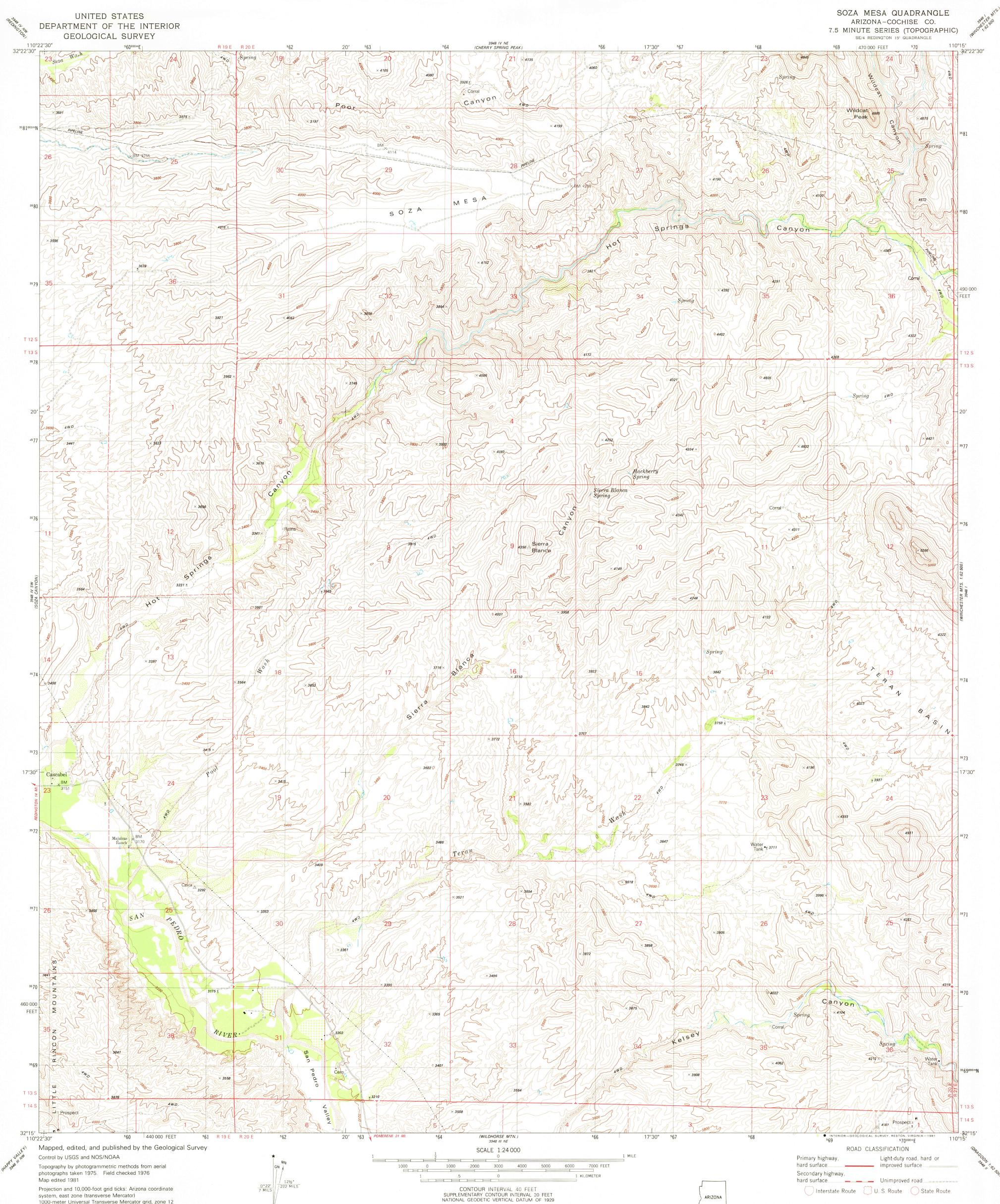
Projection and 10,000-foot grid ticks: Arizona coordinate system, east zone (transverse Mercator) 1000-meter Universal Transverse Mercator grid, zone 12 1927 North American Datum To place on the predicted North American Datum 1983 move the projection lines 6 meters south and 61 meters east as shown by dashed corner ticks
