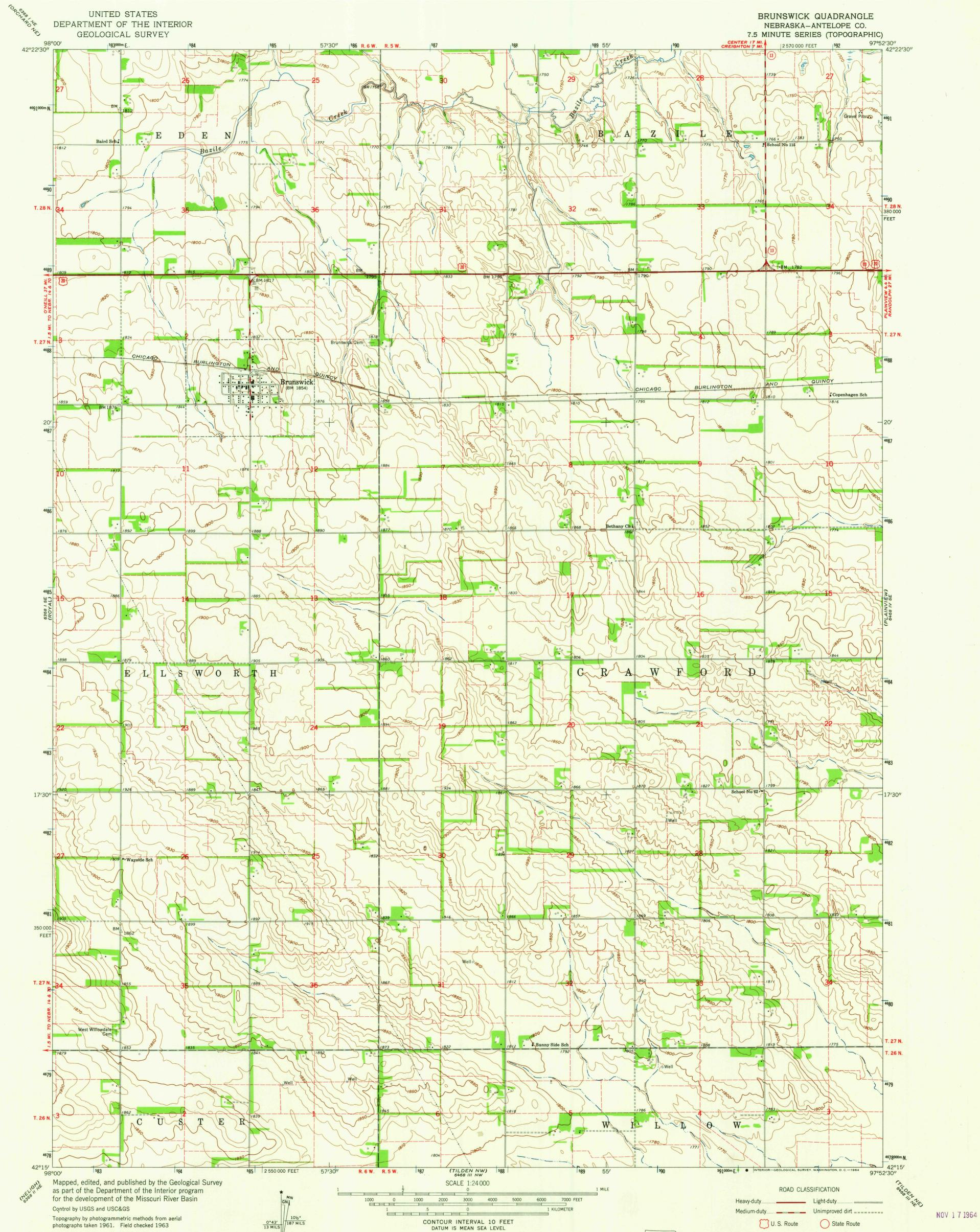
Polyconic projection. 1927 North American datum 10,000-foot grid based on Nebraska coordinate system, north zone 1000-meter Universal Transverse Mercator grid ticks, UTM GRID AND 1963 MAGNETIC NORTH DECLINATION AT CENTER OF SHEET zone 14, shown in blue
