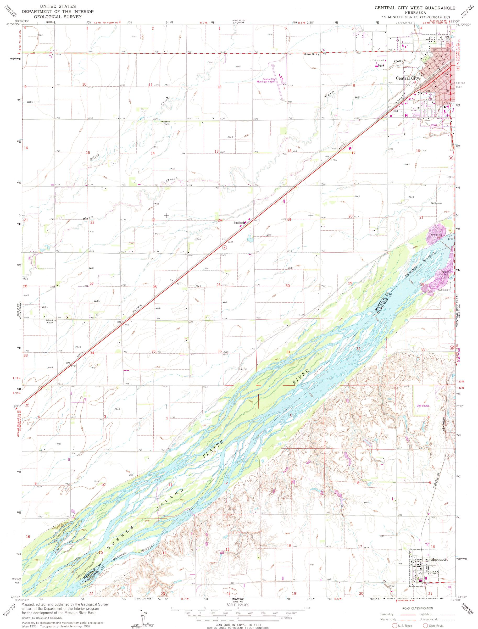
Planimetry by photogrammetric methods from aerial photographs taken 1951. Topography by planetable surveys 1962
