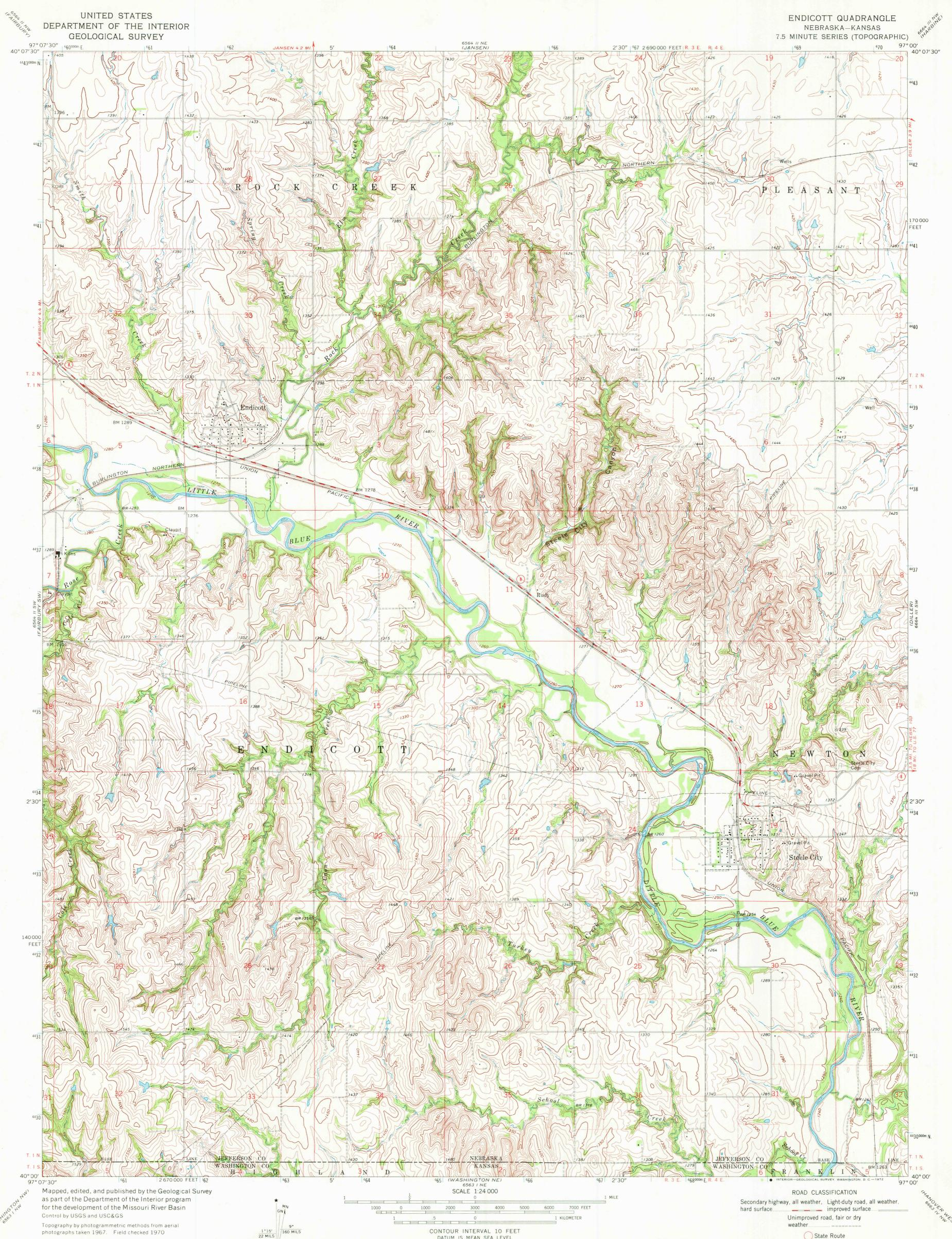
Polyconic projection. 1927 North American datum 10,000-foot grid based on Nebraska coordinate system, south zone 1000-meter Universal Transverse Mercator grid ticks, zone 14, shown in blue Fine red dashed lines indicate selected fence and field lines where
