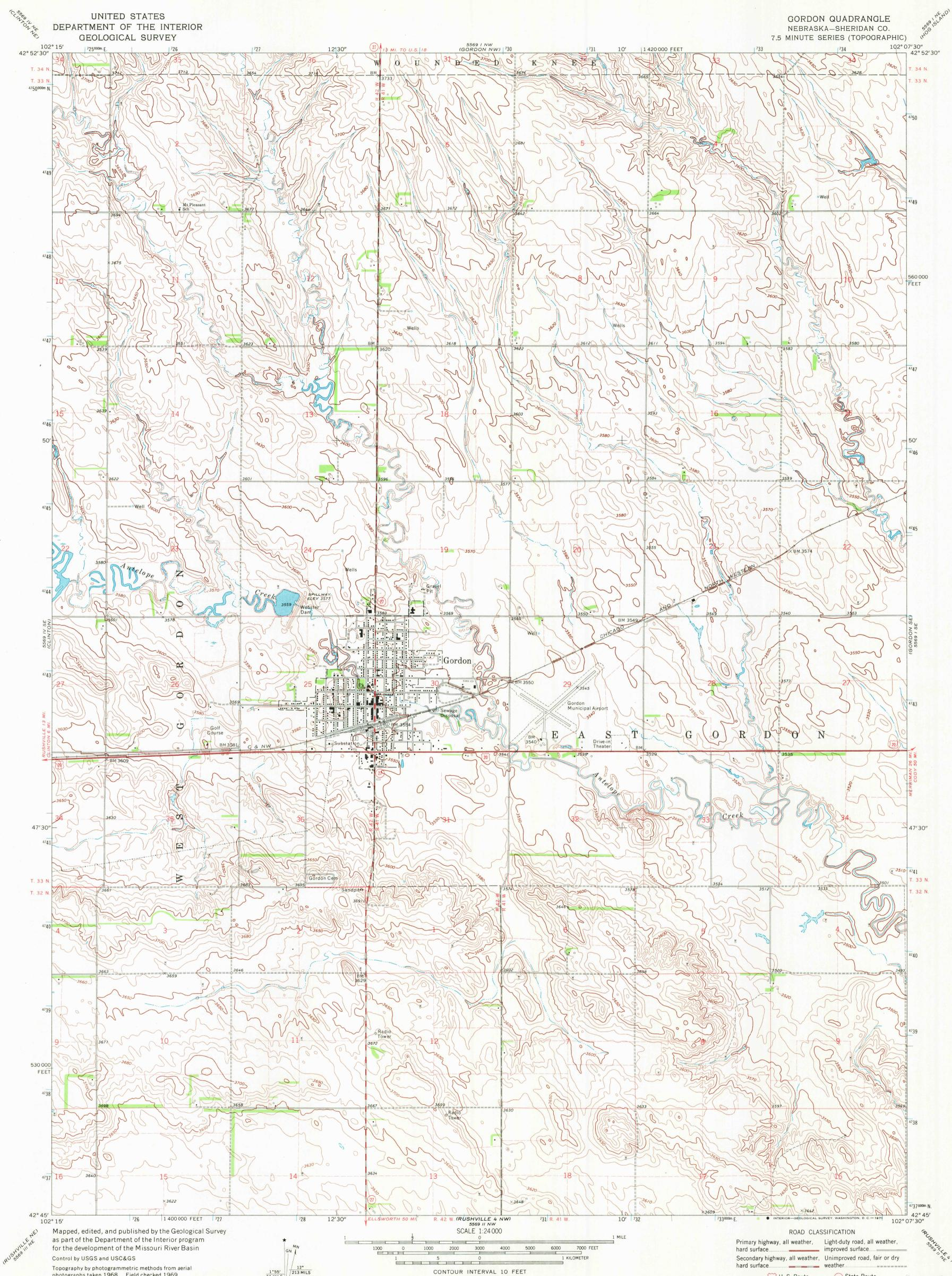
Topography by photogrammetric methods from aerial photographs taken 1968. Field checked 1969 Polyconic projection. 1927 North American datum 10,000-foot grid based on Nebraska coordinate system, north zone 1000-meter Universal Transverse Mercator grid ticks, zone 13, shown in blue
