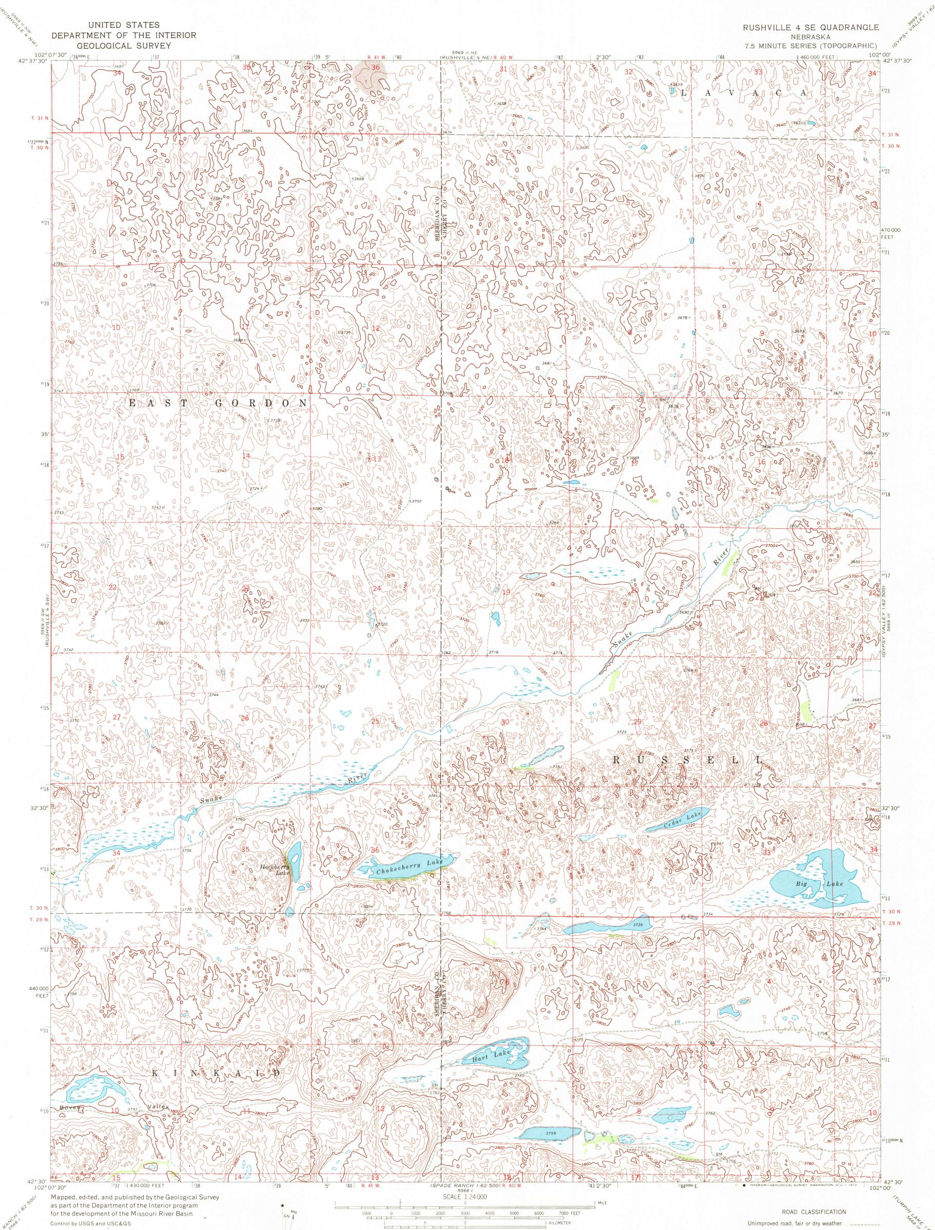
Topography by photogrammetric methods from aerial photographs taken 1968. Field checked 1969 Polyconic projection. 1927 North American datum 10,000-foot grid based on Nebraska coordinate system, north zone 1000-meter Universal Transverse Mercator grid ticks, zone 13, shown in blue
