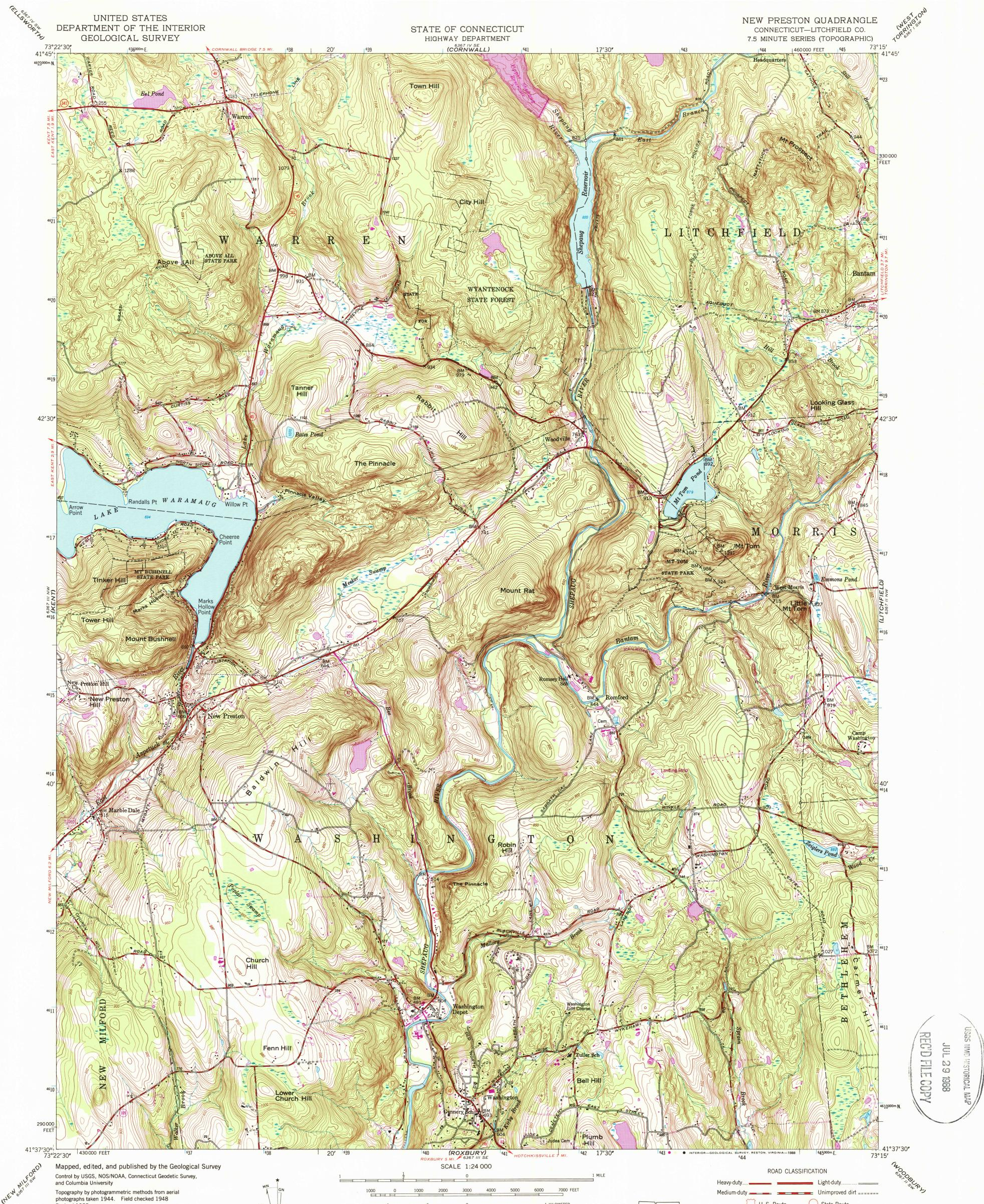
Revised 1955 Polyconic projection. 10,000-foot grid ticks based on Connecticut coordinate system 1000-meter Universal Transverse Mercator grid ticks, zone 18, shown in blue 1927 North American Datum To place on the predicted North American Datum 1983 move the projection lines 6 meters south and 37 meters west as shown by dashed corner ticks There may be private inholdings within the boundaries of the National or State reservations shown on this map
