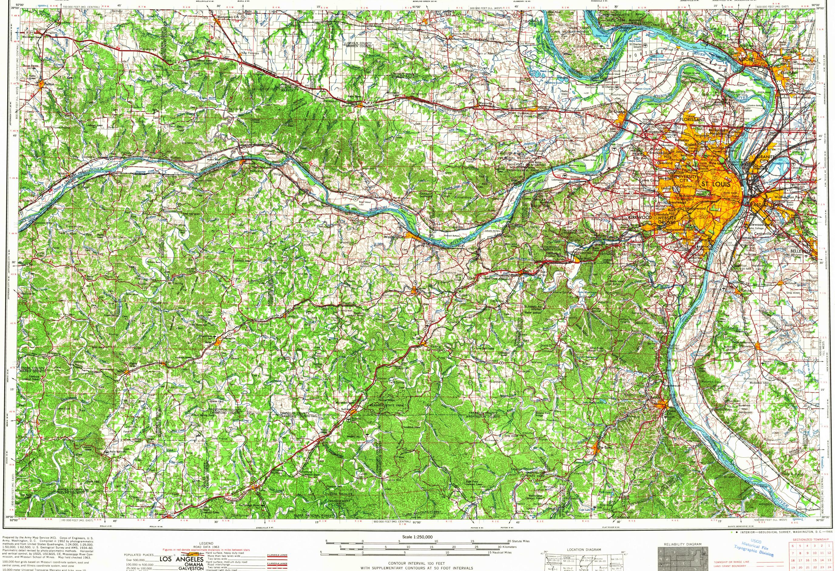
Prepared by the Army Map Service (KC). Corps of Engineers, U. S. Army, Washington, D. C. Compiled in 1962 by photogrammetric methods and from United States Quadrangles, 1:24,000, 1:25,000, 1:50,000, 1:62,500, U. S. Geological Survey and AMS, 1934–60. Planimetric detail revised by photo-planimetric methods. Horizontal and vertical control, by USGS, USC&GS, CE, Mississipppi River Commission, and Missouri School of Mines. Map field checked 1963.
