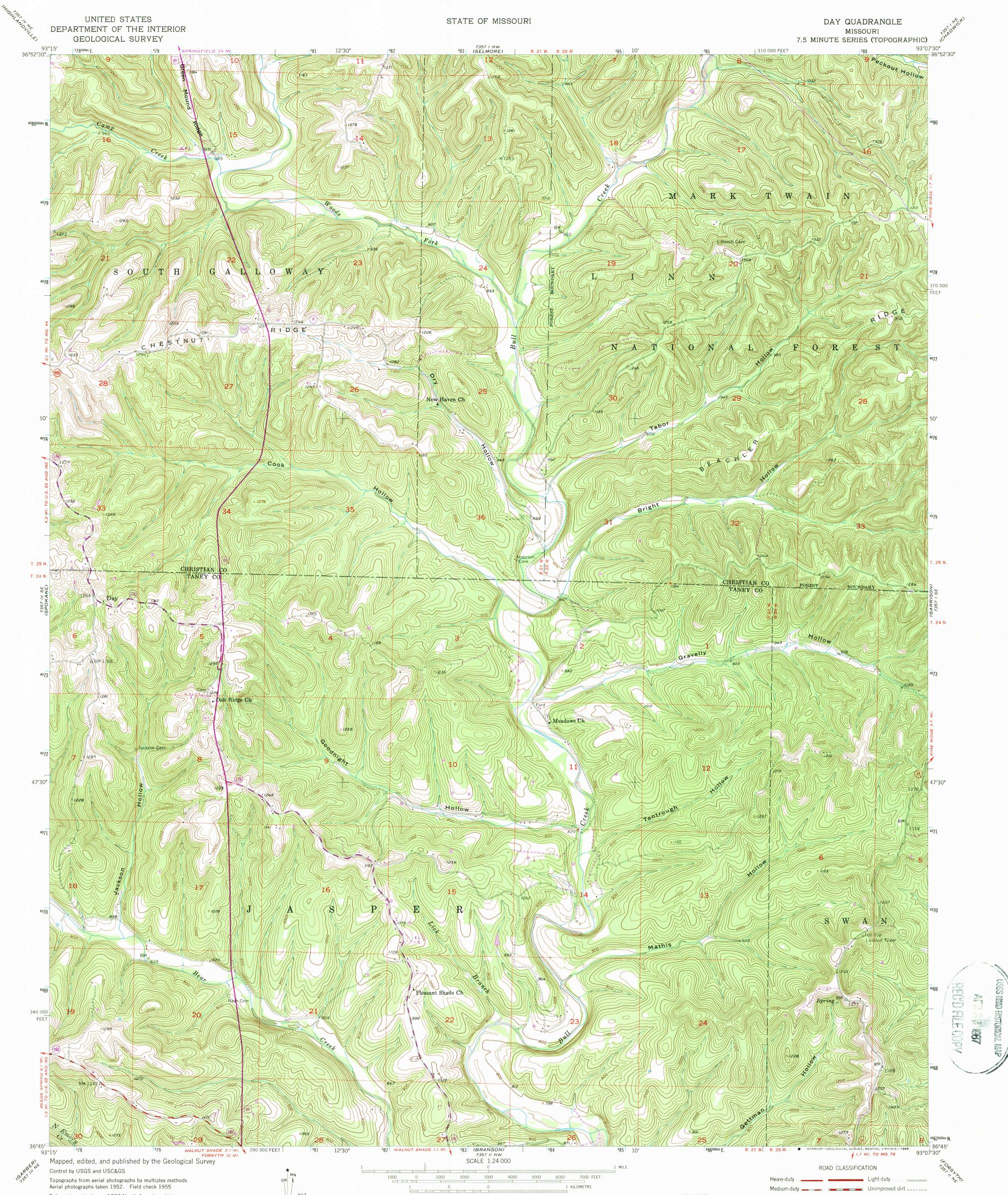
Polyconic projection. 1927 North American datum 10,000-foot grid based on Missouri coordinate system, central zone 1000-metre Universal Transverse Mercator grid ticks, zone 15, shown in blue
