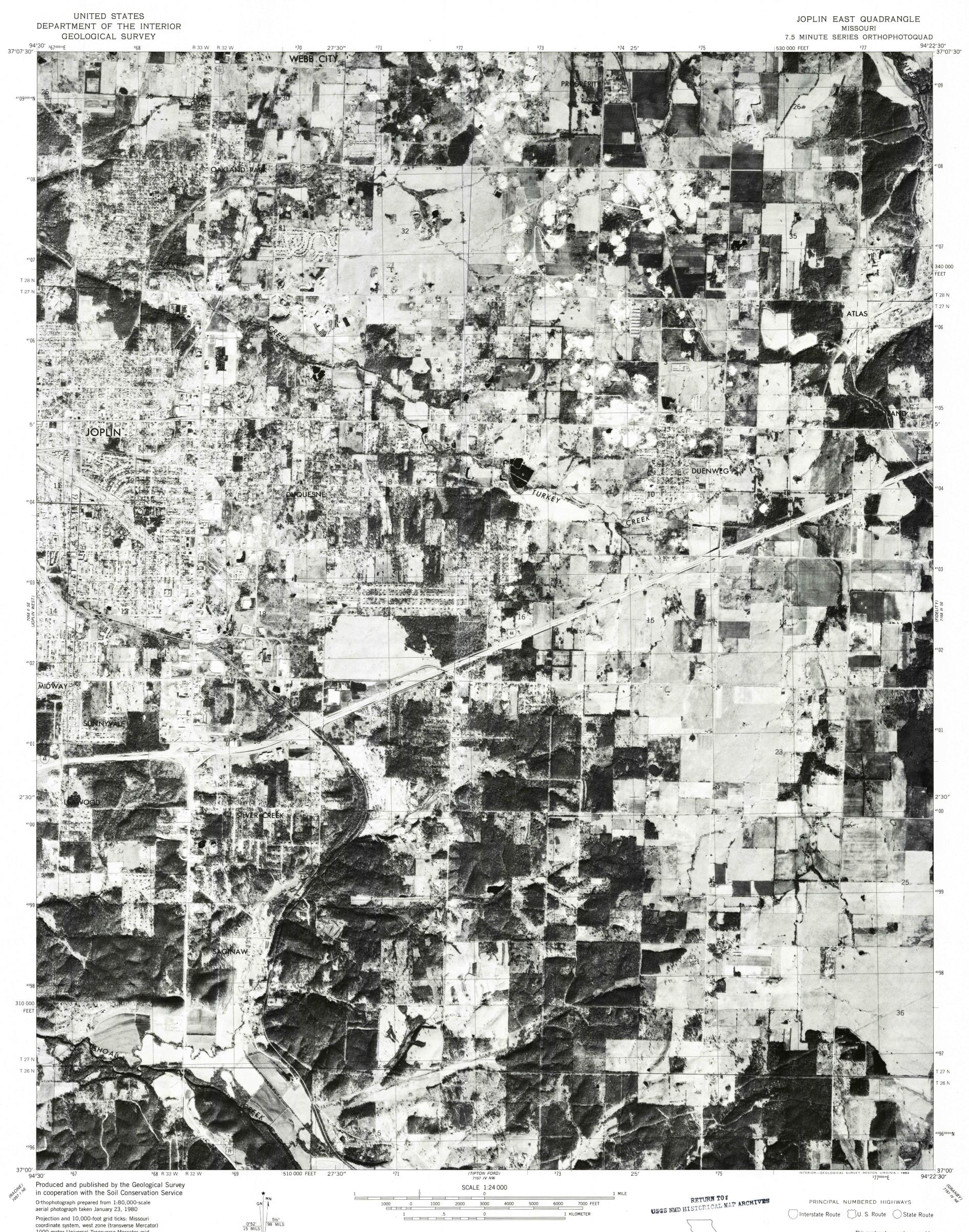
coordinate system, west zone (transverse Mercator) 1000-meter Universal Transverse Mercator grid, zone 15. 1927 North American Datum To place on the predicted North American Datum 1983 move the projection lines 3 meters south and 19 meters east as shown by dashed corner ticks Photoimagery rectified by optical scanning
