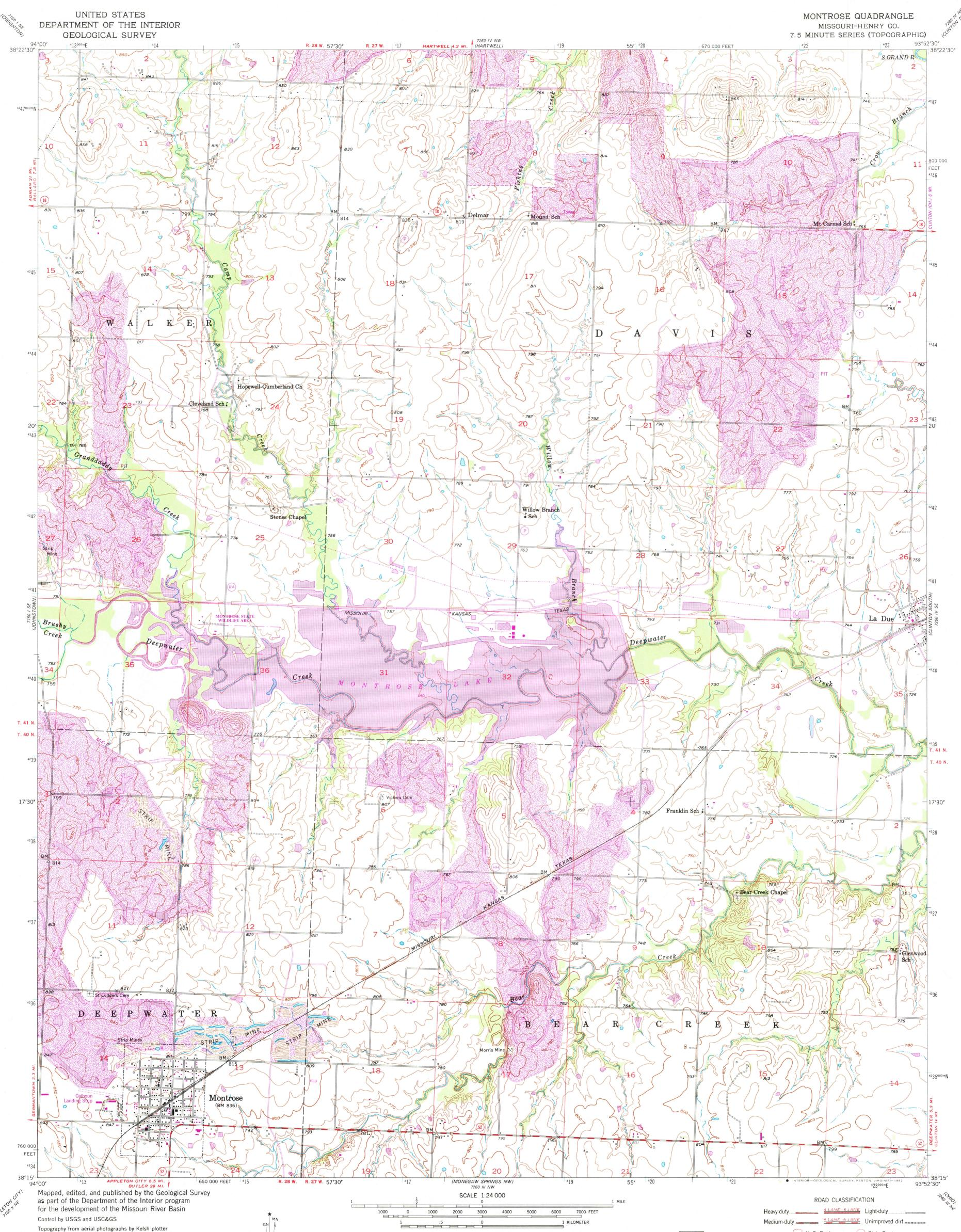
Aerial photographs taken 1951. Field check 1953 Polyconic projection. 1927 North American datum 10,000-foot grid based on Missouri coordinate system, west zone 1000-meter Universal Transverse Mercator grid ticks, zone 15, shown in blue To place on the predicted North American Datum 1983 move the projection lines 18 meters east as shown by dashed corner ticks There may be private inholdings within the boundaries of
