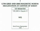
CONTOUR INTERVAL 5 FEET NATIONAL GEODETIC VERTICAL DATUM OF 1929 TO CONVERT FROM FEET TO METERS, MULTIPLY BY 0.3048
