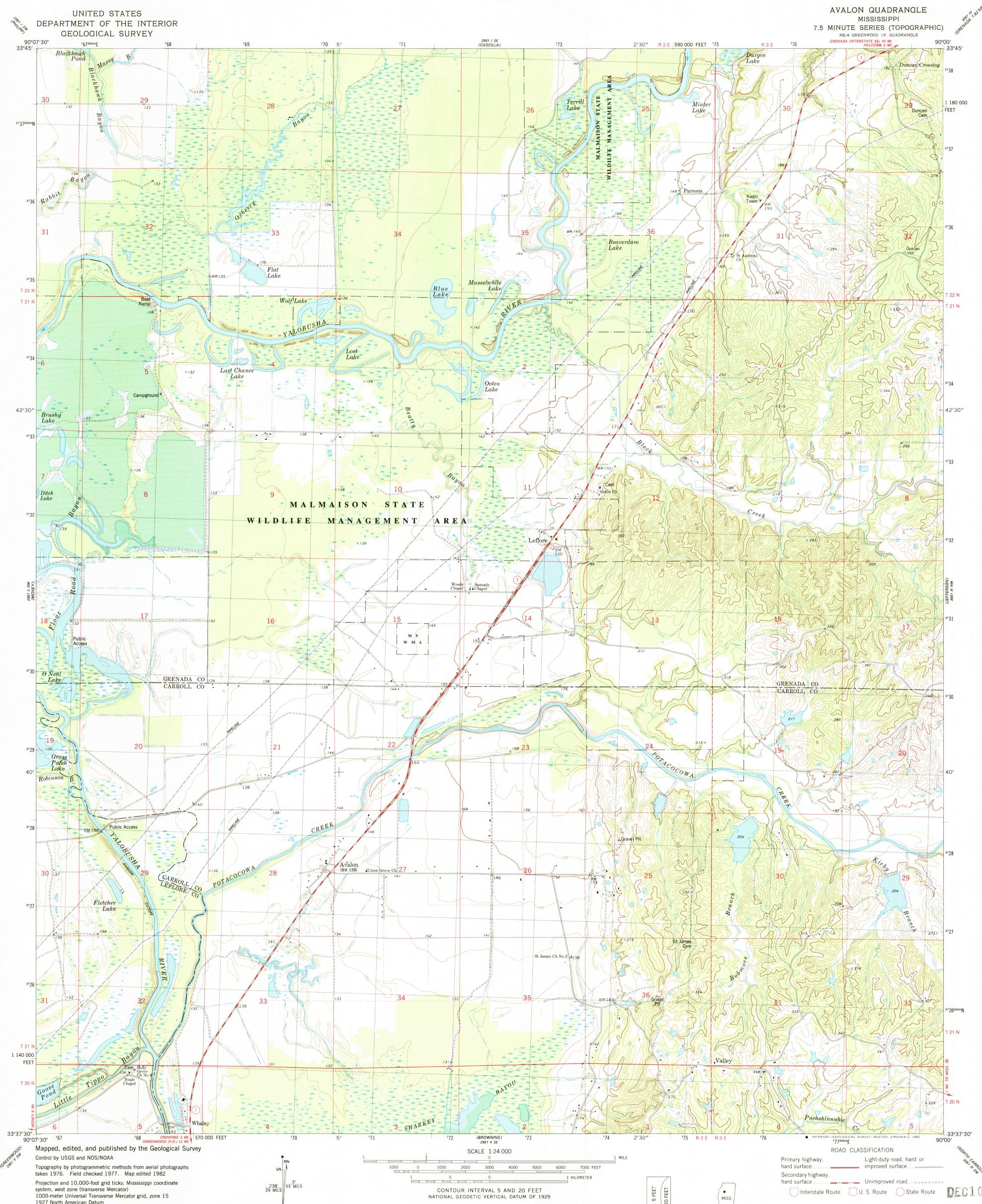
system, west zone (transverse Mercator) 1000-meter Universal Transverse Mercator grid, zone 15 1927 North American Datum To place on the predicted North American Datum 1983 move the projection lines 10 meters south and 8 meters east as shown by dashed corner ticks
