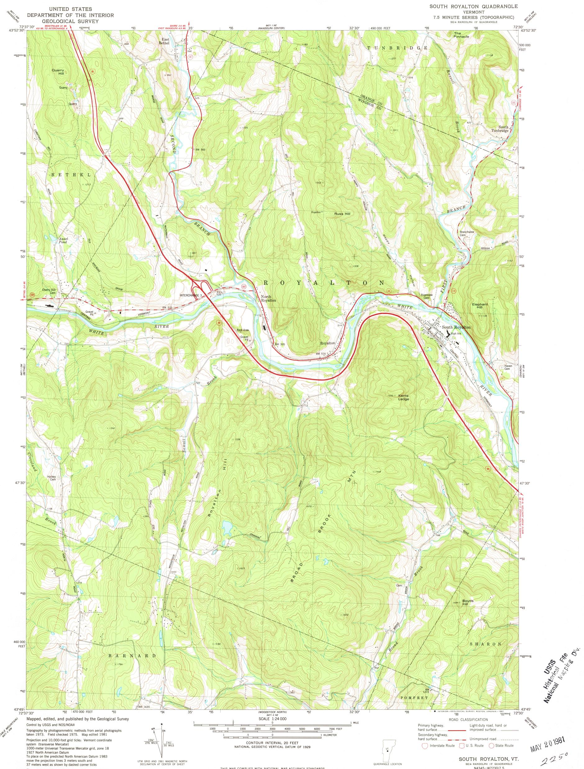
system (transverse Mercator) 1000-meter Universal Transverse Mercator grid, zone 18 1927 North American Datum To place on the predicted North American Datum 1983 move the projection lines 3 meters south and 37 meters west as shown by dashed corner ticks
