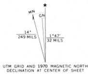
UTM GRID AND 1970 MAGNETIC NORTH DECLINATION AT CENTER OF SHEET
