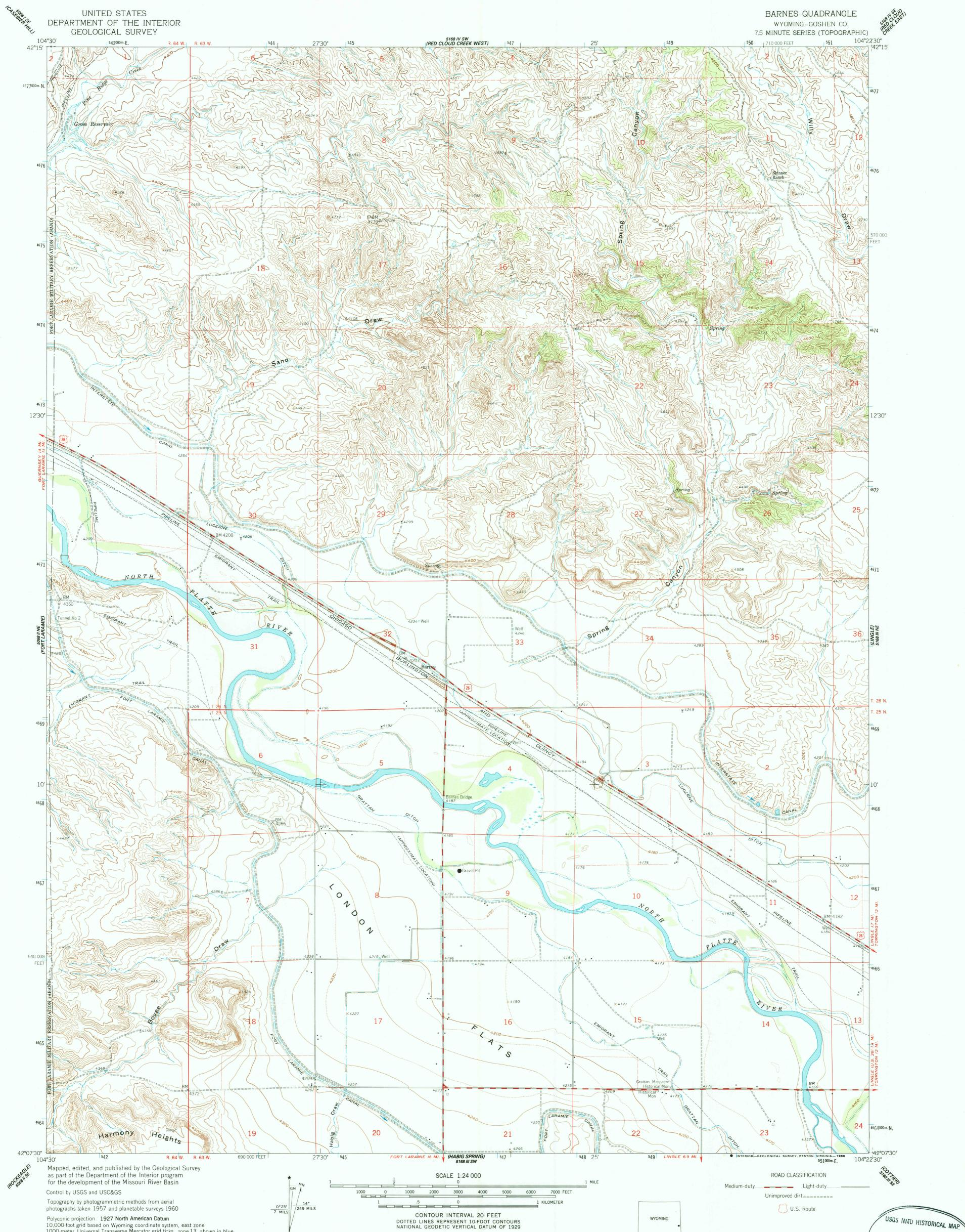
Polyconic projection. 1927 North American Datum 10,000-foot grid based on Wyoming coordinate system, east zone 1000-meter Universal Transverse Mercator grid ticks, zone 13, shown in blue
